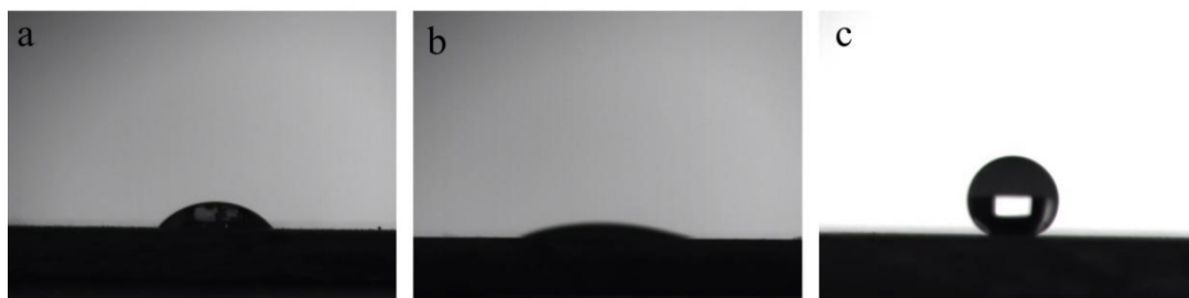
Figure 1. The CA images of (a) Mg (b) MgO/Mg and (c) PP-MgO/Mg samples
