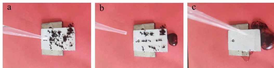
Figure 10. Self-cleaning behavior on the surface of super-hydrophobic coatings.
