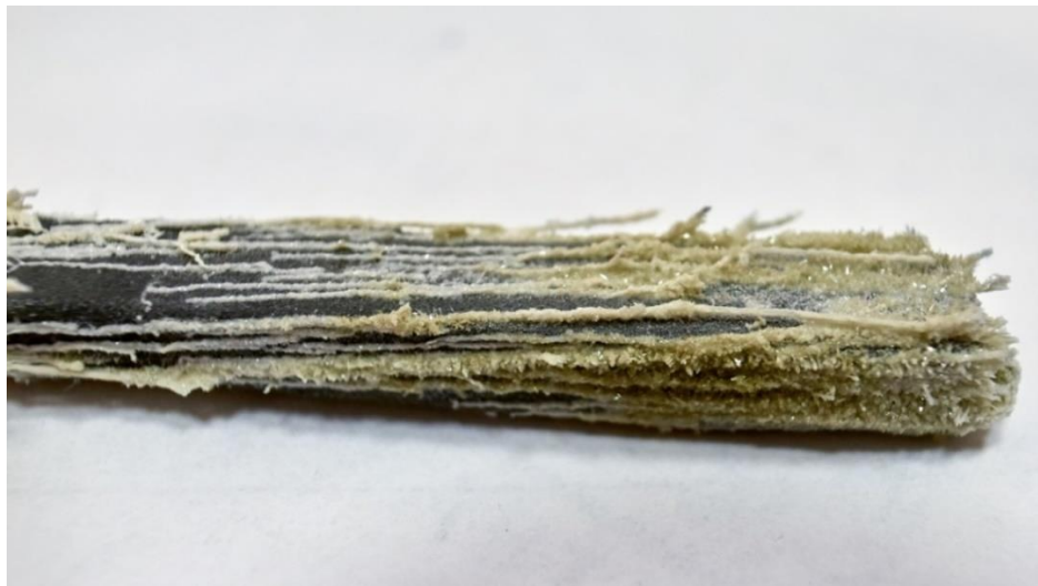
Figure 6. General view of the rhenium anode covered by the salt deposit, which was obtained at the temperature of 25°C and at the anode current density of 1 A/cm 2
