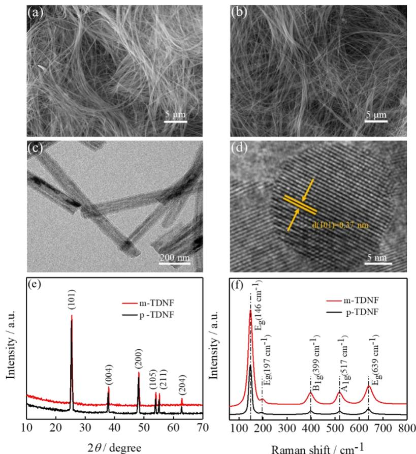
**Figure 1.** (a) SEM images of p-TDNF; (b) SEM images of m-TDNF; (c) TEM images of m-TDNF; (d)HRTEM images of m-TDNF; (e) XRD patterns, and (f) Raman spectra of the p-TDNF and m-TDNF nanoparticles.
