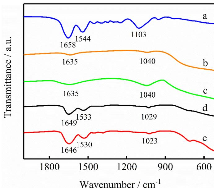
**Figure 4.** FT-IR spectra of GOD (a), p-TDNF (b), m-TDNF (c), GOD/p-TDNF (d) and GOD/m-TDNF (e).
