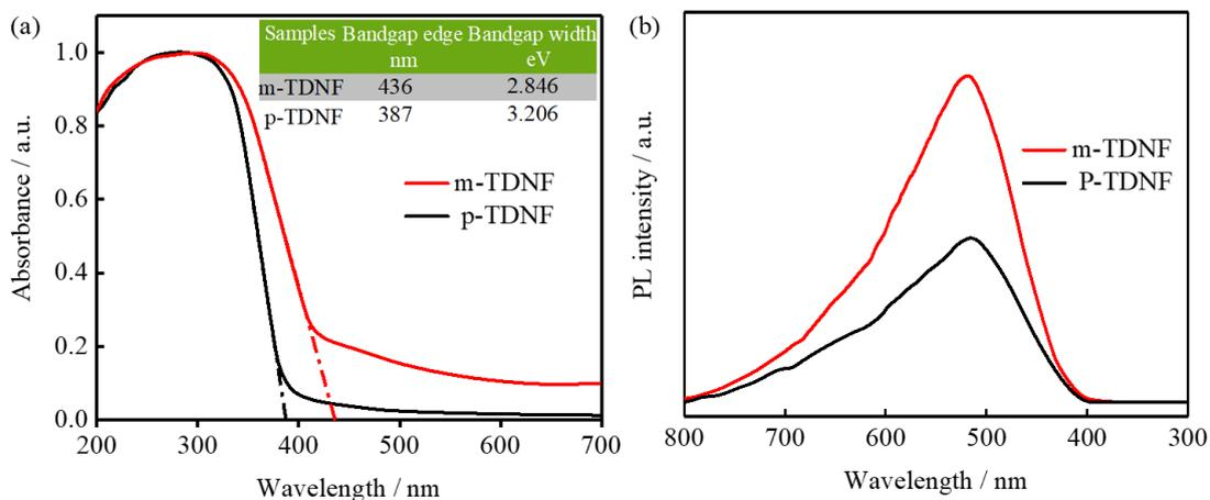
**Figure 2.** (a) UV-vis diffuse absorbance and (b) PL spectra of the p-TDNF and m-TDNF.
