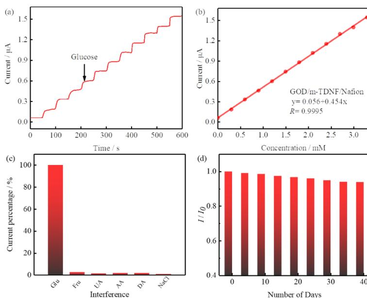
**Figure 6.** (a) Amperometric response of GOD/m-TDNF/Nafion/GCE glucose sensors in 0.1 M PBS with consecutive addition of various concentrations of glucose, (b) Linear fitting curve between current and glucose concentrations, (c) Effect of interfering species to the response and (d) Long-term stability of the GOD/m-TDNF/Nafion/GCE glucose biosensors.
