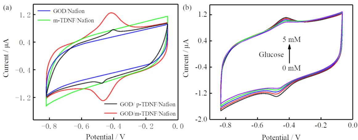
**Figure 5.** (a) CVs of GOD/Nafion/GCE, m-TDNF/Nafion/GCE, GOD/p-TDNF/Nafion/GCE and GOD/m-TDNF/Nafion/GCE in 0.1 M PBS solution (pH 7.0) at scan rate of  $100 \text{ mV s}^{-1}$ . (b) CVs of the GOD/TDNF/Nafion/GCE in 0.1 M PBS solution (pH 7.0) including 0, 0.5, 1, 2 and 5 mM glucose at a scan rate of  $100 \text{ mV s}^{-1}$ .
