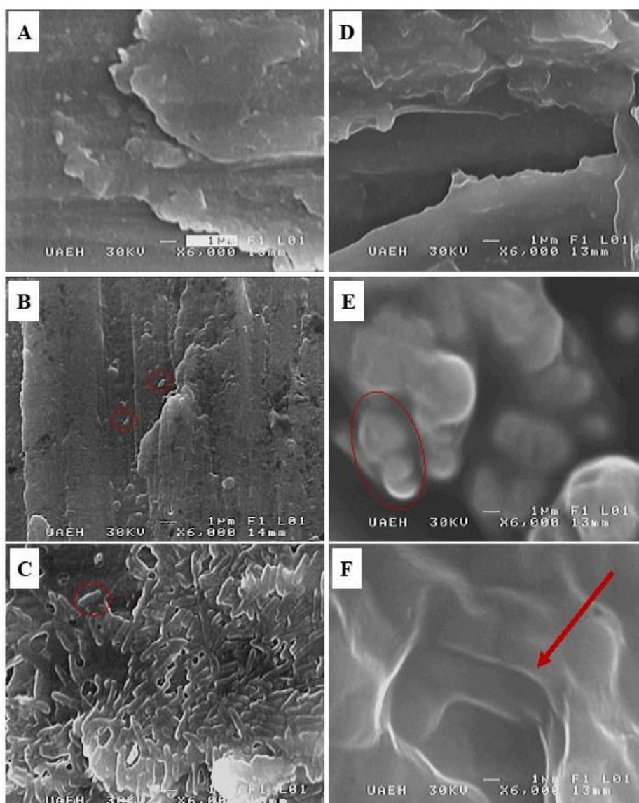
**Figure 5.** SEM micrographs of the A-Ti control electrodes (a and d) and bio-electrodes at 24 hours (b and e) and 168 hours (c and f) after the inoculation of the bacterial consortium in the biological support media PCNB (a–c) and AW (d–f).
