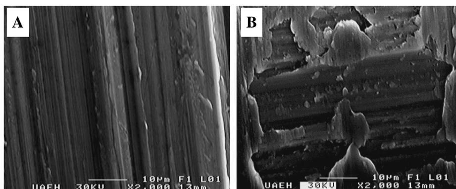
**Figure 1.** Surface scanning electron micrographs of the titanium (A) and anodised titanium (B) materials.
