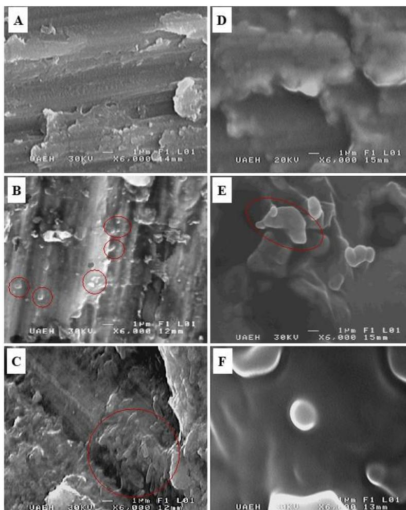
**Figure 3.** SEM micrographs of Ti electrodes, control electrodes (a and d) and bio-electrodes at 24 hours (b and e) and 168 hours (c and f) after inoculation of the bacterial consortium in biological support media PCNB (a–c) and AW (d–f).
