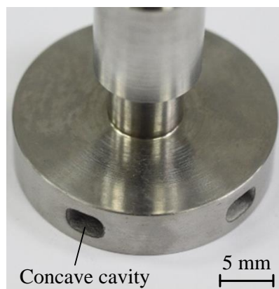
Figure 6. Cylindrical cathode tool used in CRECM.
