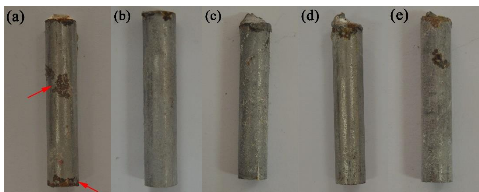
Figure 9. Photographs of carbon steel samples in chloride contaminated mortar with different concentrations of SPP at 90 d. (a) 0%, (b) 0.3%, (c) 0.6%, (d) 1.2%, (e) 2.4%.
