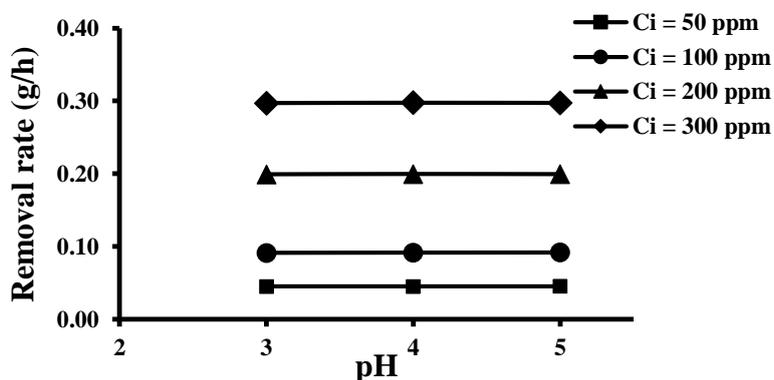
Figure 8. Effect of pH on removal rate at different initial concentrations, a current density of 0.98 mA/cm<sup>2</sup> and a flow rate of 0.278 ml/s.
