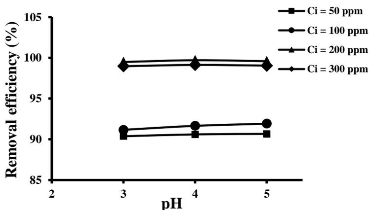
Figure 9. Effect of pH on removal efficiency at different initial concentrations, a current density of 0.98 mA/cm<sup>2</sup> and a flow rate of 0.278 ml/s.
