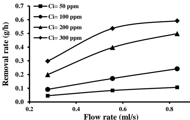
**Figure 5.** Effect of feed flow rate on removal rate at a constant current density of 0.98 mA/cm<sup>2</sup> and pH 4.
