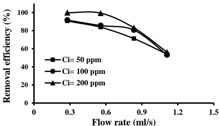
**Figure 4.** Effect of feed flow rate on removal efficiency at different initial concentrations, a current density of 0.98 mA/cm<sup>2</sup> and pH 4.
