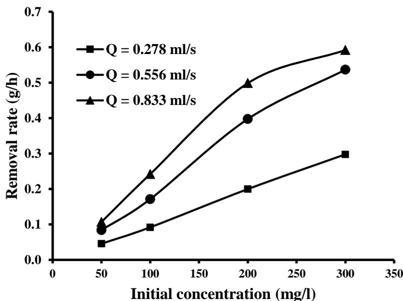
**Figure 3.** Effect of initial concentration on removal rate at different flow rates, a current density of 0.98 mA/cm<sup>2</sup> and pH 4.
