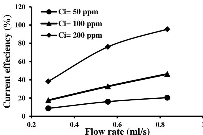
**Figure 6.** Effect of flow rate on current efficiency at a current density of 0.98 mA/cm<sup>2</sup> and pH= 4.
