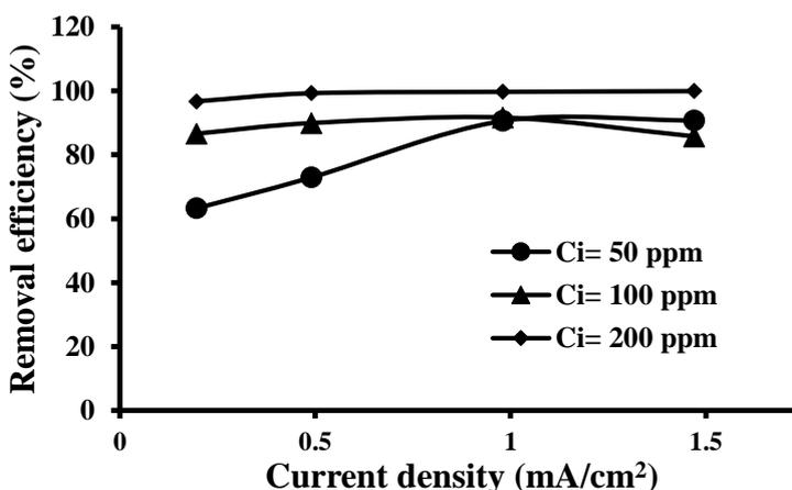
**Figure 7.** Effect of current density on removal efficiency at a flow rate of 0.278 ml/s and pH 4.
