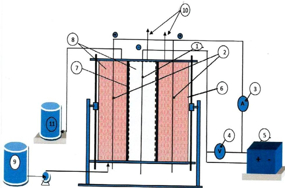
**Figure 1.** Schematic of the experimental setup: 1) anode current collector; 2) cathode current collector; 3) ammeter; 4) voltmeter; 5) DC power supply; 6) Plexiglas cylinder; 7) stainless steel cylinder; 8) graphite; 9) iron solution tank; 10) gas vents; 11) treated water tank; 12) dosing pump.
