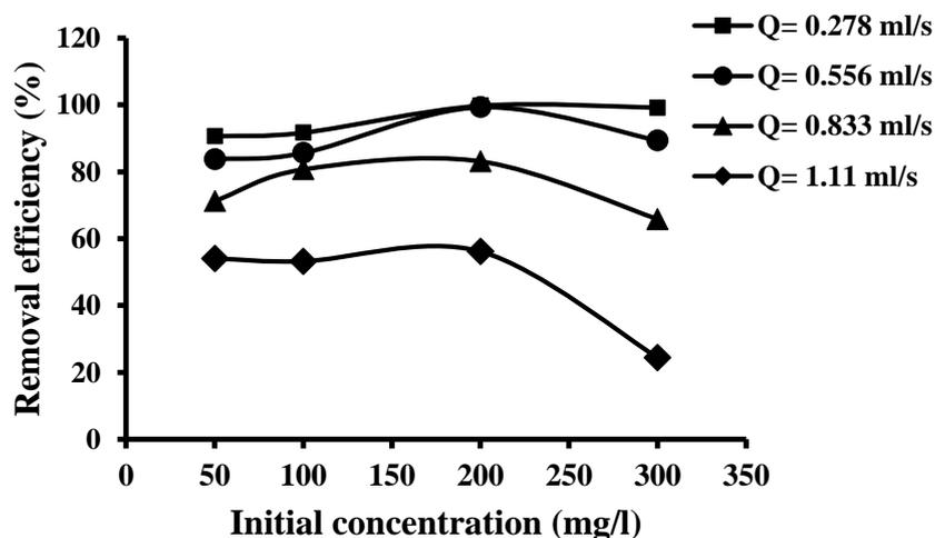
**Figure 2.** Effect of initial concentration on removal efficiency at different flow rates, a current density of  $0.98 \text{ mA/cm}^2$  and  $\text{pH} = 4$ .
