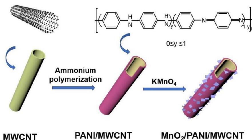
**Figure 1.** The fabrication procedure for the ternary nanocomposite  $MnO_2$ /PANI/MWCNTs.
