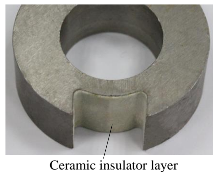
Figure 12. Photograph of tool electrode with concave cavity.
