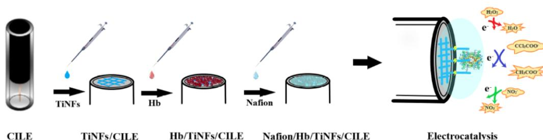
**Scheme 1.** Construction process of Nafion/Hb/TiNFs/CILE and its electrocatalysis
