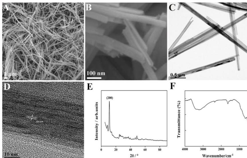
**Figure 1.** SEM (A, B), TEM (C), HRTEM (D), XRD (E) and FT-IR spectrum (F) of TiNFs
