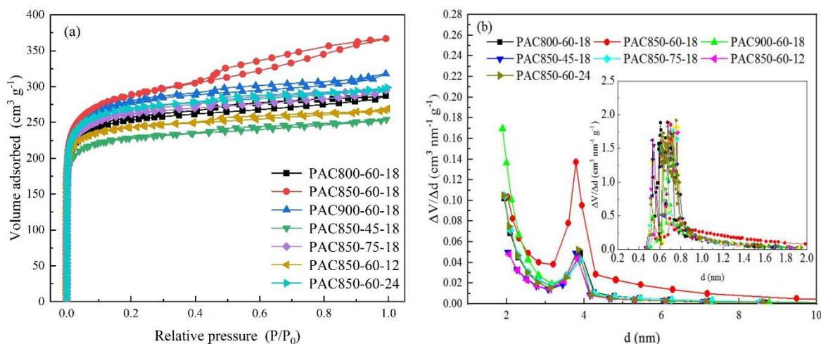
**Figure 2.** (a) Nitrogen adsorption-desorption isotherms and (b) mesopore pore size distribution of PAC (the inset shows the pore size distribution of the micropore).
