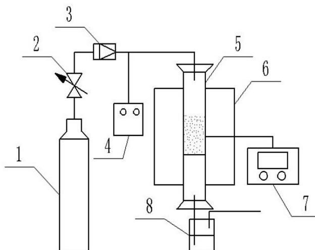
1. Nitrogen cylinder 2.Compression release valve 3. Gas flow indicator 4.Liquid flowmeter 5.Quartz reaction tube 6.Heating electric furnace 7.Digital display temperature controller 8.Exhaust gas treatment
