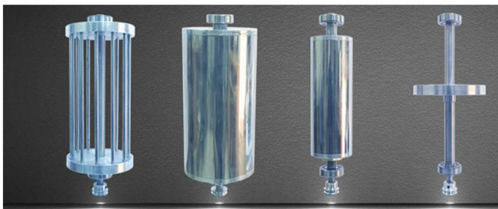
Figure 3. Different collectors for electrospinning. This figure has been republished with permission of an open-access article of Springerlink.com, from [Review for application of electrospinning and electrospun nanofibers technology in textile industry, M. Mirjalili, S. Zohoori, Journal of Nanostructure in Chemistry , 6, 207-213, 2016.].
