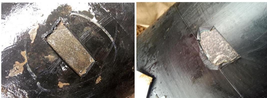
**Figure 1.** Pictures of delaminated coating without defects in field
