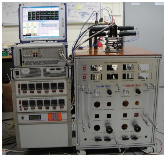
Figure 15. PEM electrolyzer test station built in PSSEL laboratory of INJE University.
