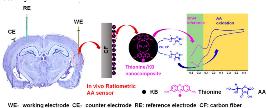
Figure 7. Schematic illustration of rationally designed ratiometric electrochemical sensor for selective and reliable measurement of cerebral AA in living brains. Reprinted with permission from reference [55]. Copyright 2017 American Chemical Society.
