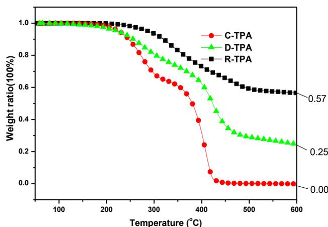
**Figure 2.** TGA thermograms of **C-TPA**, **D-TPA**, and **R-TPA**
