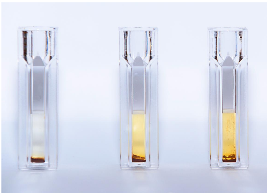
Figure 1. An example of pseudoperoxidase reaction by magnetic particles located on the bottom of a standard 1 ml cuvette. The reaction is manifested by yellow color provided by o -phenylenediamine dihydrochloride in the presence of hydrogen peroxide (increasing concentration in the cuvettes from left to right). The picture comes from author's unpublished experiments.
