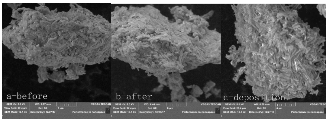
Figure 7. a Surface change of soil particles before, b after in electrokinetic remediation and c deposition in the cathode wells
