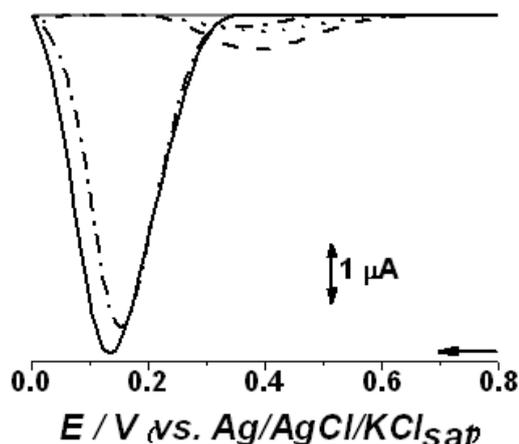
**Figure 3.** DP voltammograms obtained for 100  $\mu\text{M}$  catechol solution at CPE (●●●),  $\text{TiO}_2\text{@CPE}$  (—),  $\text{Lcc@CPE}$  (---) and  $\text{Lcc-TiO}_2\text{@CPE}$  (—) all in 0.1 M PBS (pH 7.0).
