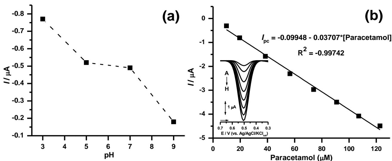
**Figure 5.** (a) pH response study for Lcc-TiO<sub>2</sub>@CPE. (b) Calibration curve obtained from DPVs in 0.1 M PBS (pH 3.0), for increasing concentrations (A) 10 to (H) of paracetamol.
