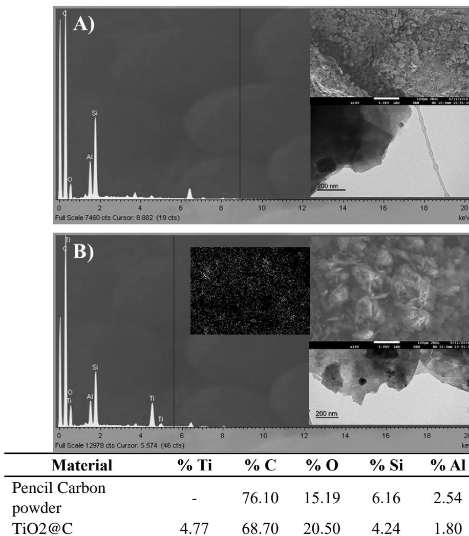
**Figure 1.** EDX spectrum with SEM TEM imagens: **A)** unmodified pencil powder **B)** TiO<sub>2</sub>@C powder. In addition, table with EDX elementary results.
