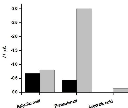
**Figure 4.** Response to  $\text{TiO}_2\text{@CPE}$  (black) and  $\text{Lcc-TiO}_2\text{@CPE}$  (light grey) in the analysis of different analytes, at 100  $\mu\text{M}$  concentration in 0.1 M PBS (pH 7.0).
