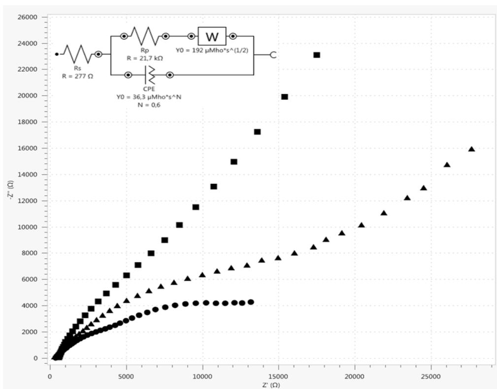
**Figure 2.** Nyquist plots obtained for: (squares) CPE, (triangles) Lcc-TiO<sub>2</sub>@CPE and (circles) TiO<sub>2</sub>@CPE. **Insert.** Equivalent electrical circuit for Lcc-TiO<sub>2</sub>@CPE, presenting the solution resistance ( $R_s$ ), the polarization resistance ( $R_p$ ), the Warburg impedance (W) and the capacitance of the system (Constant Phase Element = CPE).
