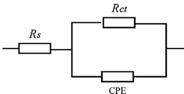
**Figure 4.** Equivalent circuit model used to fit the EIS experiment data.
