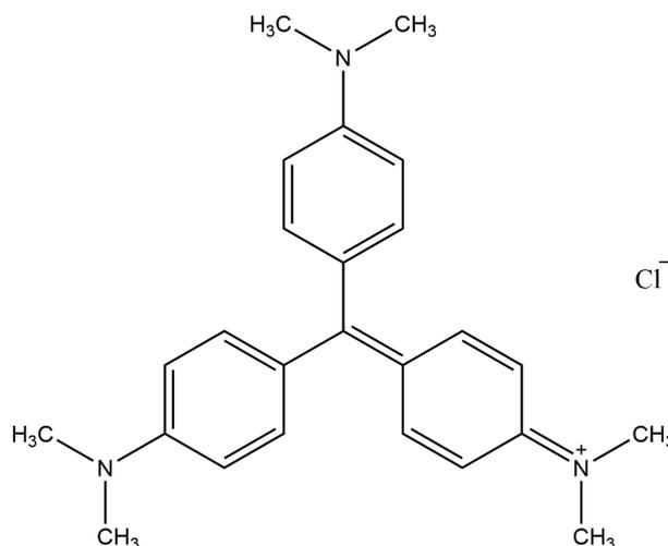
**Figure 1.** Structure of MV
