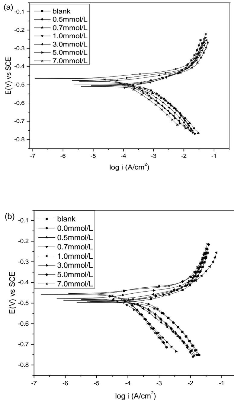
**Figure 2.** Potentiodynamic polarization curves of carbon steel containing different concentrations of I<sup>-</sup> without (a) and with (b) 0.4 mmol/L MV in the 1.0 mol/L  $\text{H}_3\text{PO}_4$  at 40°C.
