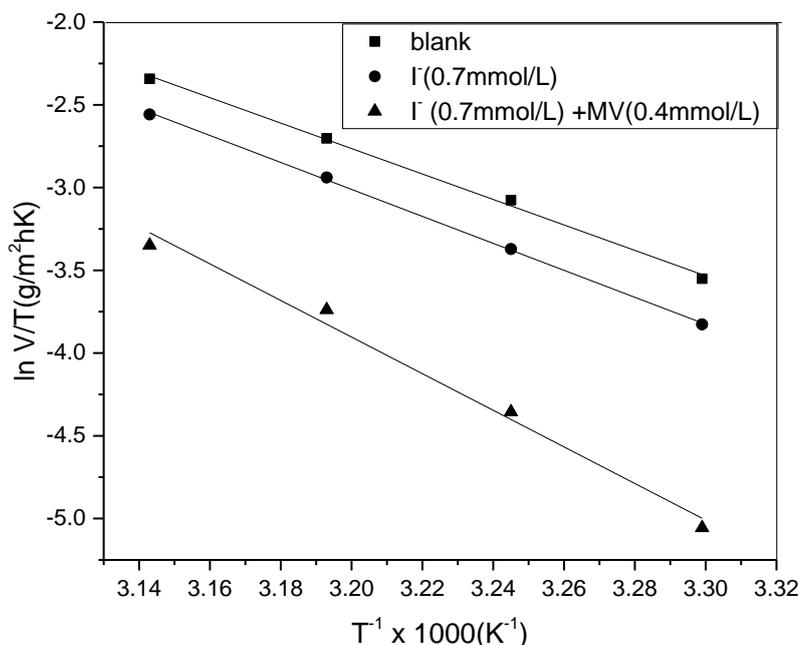
**Figure 6.** Transition state plots of the carbon steel in 1.0 mol/L H<sub>3</sub>PO<sub>4</sub>.
