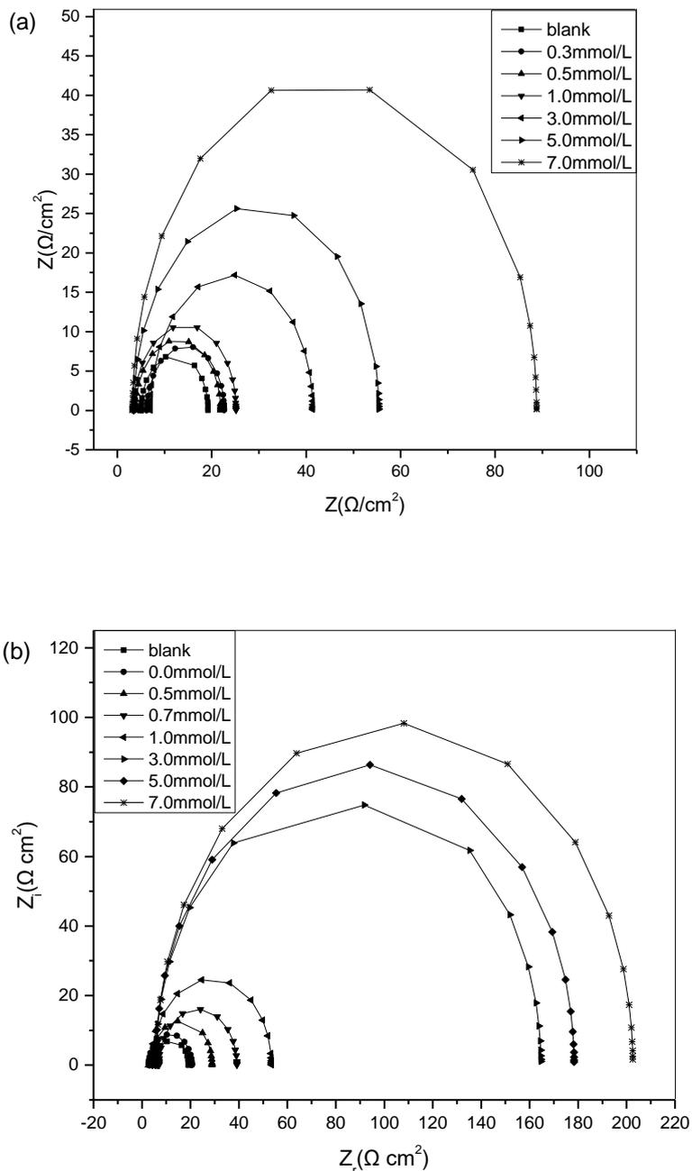
**Figure 3.** Nyquist plots of the carbon steel containing different concentrations of  $I^-$  without (a) and with (b) 0.4 mmol/L MV in the 1.0 mol/L  $H_3PO_4$  at 40°C.
