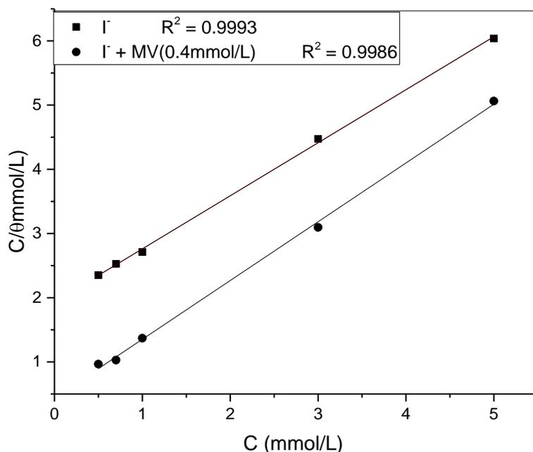
**Figure 7.** The plot of  $C/\theta$  against  $C$  in 1.0 mol/L  $H_3PO_4$  at 40°C.
