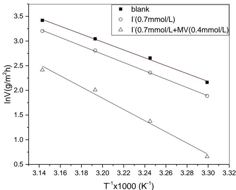
**Figure 5.** Arrhenius plots of the carbon steel in 1.0 mol/L  $H_3PO_4$ .
