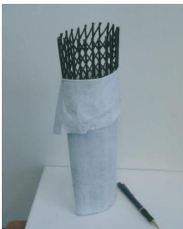
**Figure 1.** View of the electrokinetic geosynthetic material used in the Fourie [36] study.
