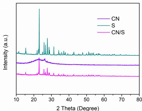
**Figure 4.** The XRD patterns of carbon nanofiber, sulfur and CN/S composite at 2 theta from  $10^{\circ}$  to  $80^{\circ}$ .
