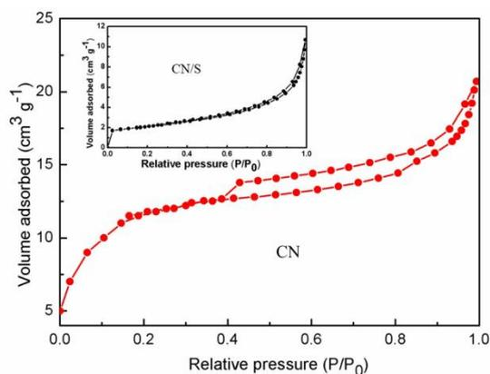
**Figure 2.** The nitrogen adsorption–desorption isotherms of CN and CN/S composite.
