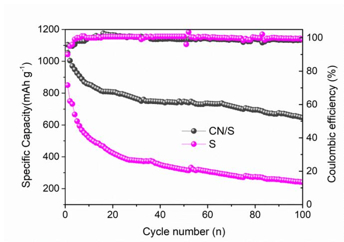
**Figure 6.** The cycle performance of pure sulfur and CN/S composite for 100 cycles at the current density of 0.2 C.
