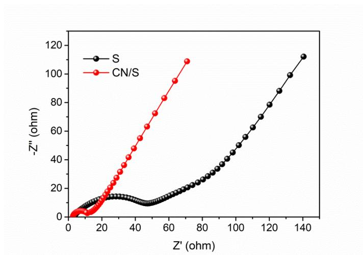
**Figure 8.** The EIS spectra of pure sulfur and CN/S composite.
