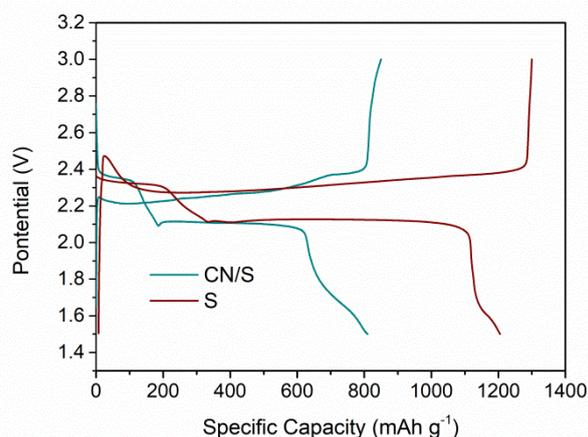
**Figure 5.** The first charge-discharge profiles of pure sulfur and CN/S composite at the current density of 0.1 C between 1.5 V and 3.0 V.
