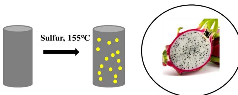
**Figure 1.** The schematic for the preparation of CN/S composites.
