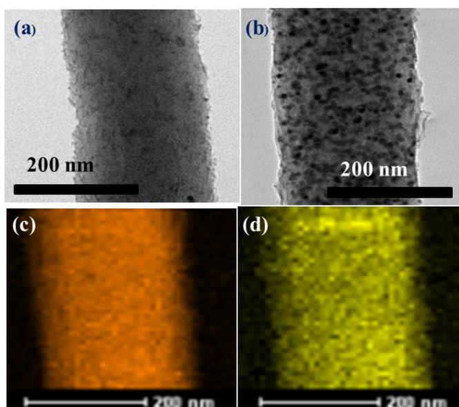
**Figure 3.** The TEM images of (a) carbon nanofiber (CN), (b) CN/S composite, (c-d) corresponding elemental mapping of CN/S composite.
