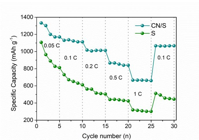
**Figure 7.** The rate performance of pure sulfur and CN/S composite at various current densities from 0.05 C to 1 C.
