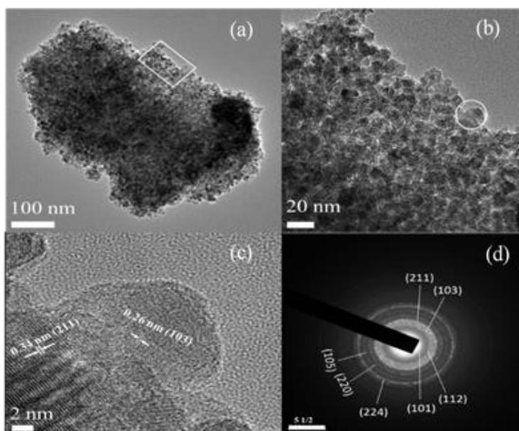
**Figure 2:** TEM images of a) a specific microparticle b) high-magnification TEM image of the selected portion in image (a), as indicated by the box, c) HRTEM image of selected nanoparticle,
