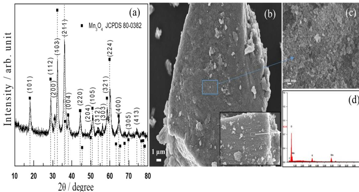
**Figure 1.** (a) XRD pattern and (b) SEM image of a selected microparticle (the inset is a magnified FESEM image of another specific particle). (c) High-magnification SEM image captured at the selected portion of a microparticle (marked with the colored box in Fig. 1b); the inset shows a cross-sectional SEM image of the microparticle. (d) EDX elemental mapping of the selected area marked by the white box shown in the inset in Fig. 1b.
