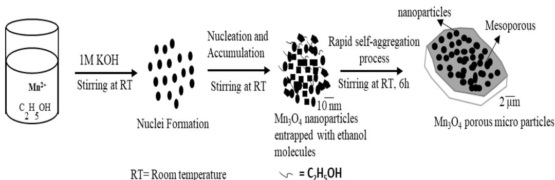
**Scheme 1.** Schematic representation of the synthesis of Mn<sub>3</sub>O<sub>4</sub> porous microstructures.
