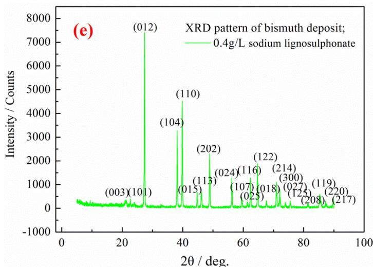
**Figure 5.** XRD patterns of bismuth deposits obtained from HCl-NaCl-BiCl<sub>3</sub> solution with different added concentrations of SLS: (a) blank, (b) 0.1 g/L, (c) 0.2 g/L, (d) 0.3 g/L, (e) 0.4 g/L.
