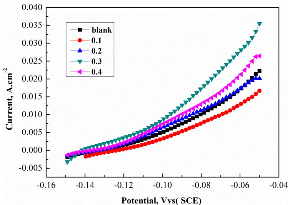
**Figure 2.** Effects of SLS concentration on cathodic polarization for bismuth electrodeposition from HCl-NaCl-BiCl<sub>3</sub> solution.
