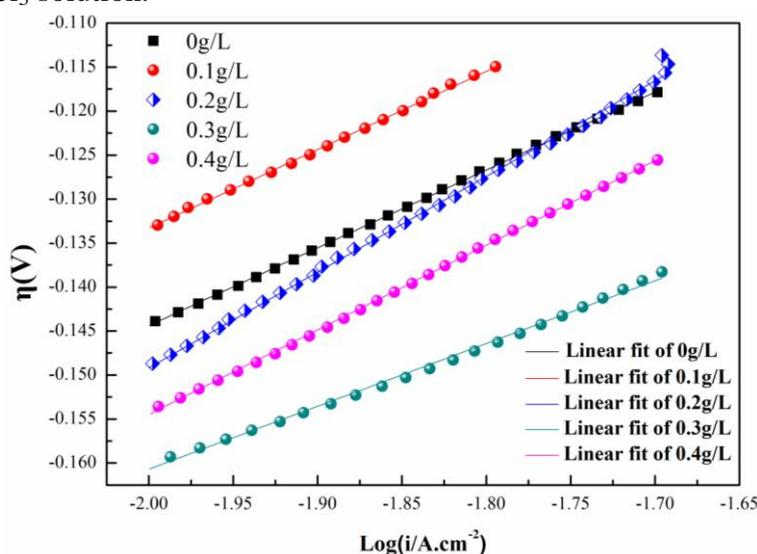
**Figure 3.** Plots of overpotential vs. the logarithm of current density for bismuth electrodeposition from HCl-NaCl-BiCl<sub>3</sub> solution
