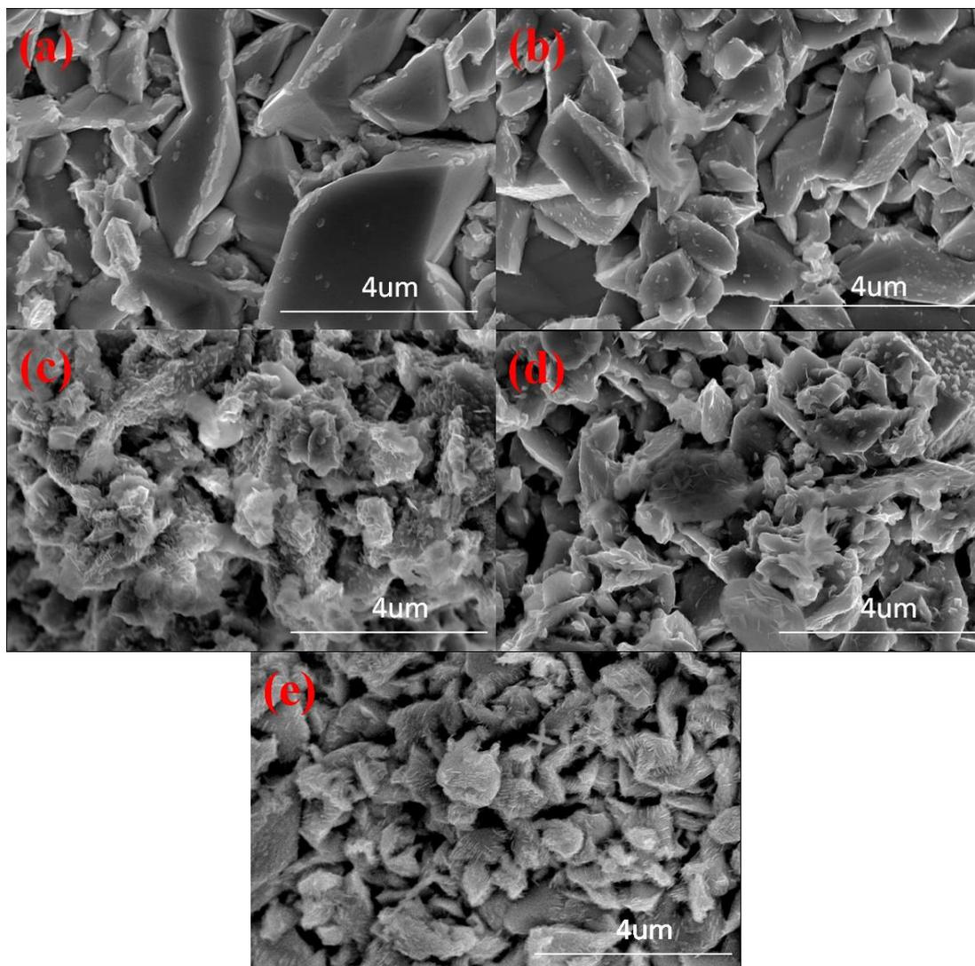
**Figure 4.** Scanning electron microscopy photomicrographs ( $\times 40000$ ) of bismuth deposits obtained from different bath solutions with different added concentrations of SLS: (a) blank, (b) 0.1 g/L, (c) 0.2 g/L, (d) 0.3 g/L, and (e) 0.4 g/L.
