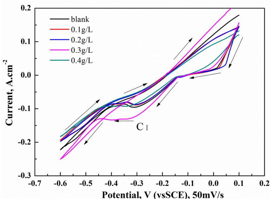
**Figure 1.** Cyclic voltammograms of copper electrodes in HCl-NaCl-BiCl<sub>3</sub> solutions with different sodium lignosulfonate (SLS) concentrations. The SLS concentration varied from 0.0 to 0.4 g/L (scan rate, 50 mV/s).
