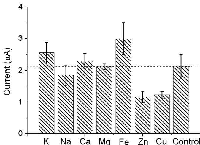
**Figure 3.** Peak currents of Cd<sup>2+</sup> in the presence and absence of foreign ions (Ca<sup>2+</sup>(100 times), K<sup>+</sup>(2000 times), Na<sup>+</sup>(100 times), Mg<sup>2+</sup>(500 times), Fe<sup>3+</sup>(20 times), Zn<sup>2+</sup>(30 times), Cu<sup>2+</sup>(4 times))
