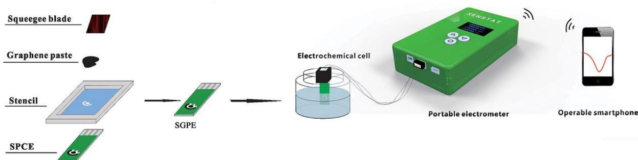
**Scheme 1.** Scheme of the fabrication of SGPE by screen-printing and DPV performed on SGPE
