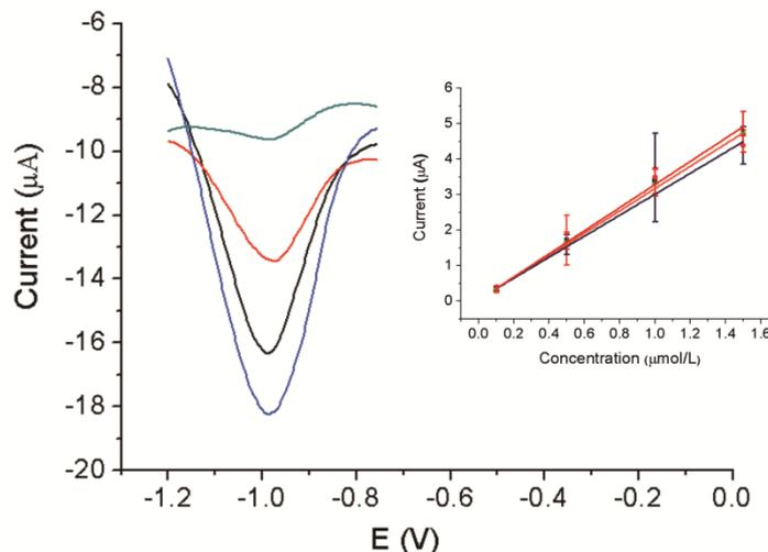
**Figure 4.** The DPV curves of different concentrations of  $\text{Cd}^{2+}$  at CHI, insert: standard addition curves of three rice samples ( $n=5$ )
