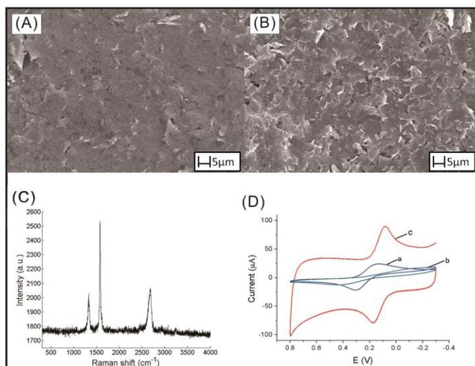
**Figure 1.** SEM images of SPCE(A) and SGPE(B), Raman spectrum of SGPE(C) and cyclic voltammograms of glass carbon electrode vs  $\text{Hg}/\text{HgCl}_2$  (a), SPCE(b) and SGPE(c) vs  $\text{Ag}/\text{AgCl}$  in  $2\text{ mmol/L K}_3\text{Fe}(\text{CN})_6$  (D)
