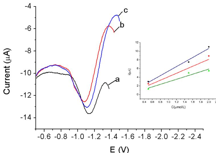
**Figure 5.** The DPV curves of 0.5(a), 1.5(b) and 2 μmol/L(c) Cd<sup>2+</sup> at Xenstat, insert: standard addition curves of three rice samples
