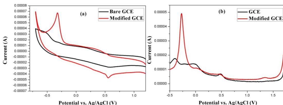
**Figure 3.** CV (a) and DPV (b) of  $2.84 \times 10^{-4}$  M 4-NP in 1 M  $\text{H}_2\text{SO}_4$  for bare GCE and TLISS/GCE
