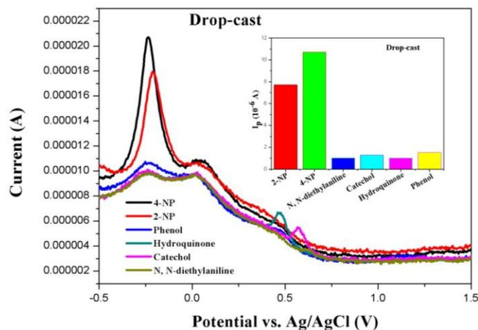
**Figure 4.** DPV diagrams and peak current ( $I_p$ ) of 4-NP, 2-NP, phenol, catechol, N,N-diethylaniline and hydroquinone in 1 M  $H_2SO_4$  for TLISS/GCE (The concentration of all the substances were  $2.84 \times 10^{-4}$  M)
