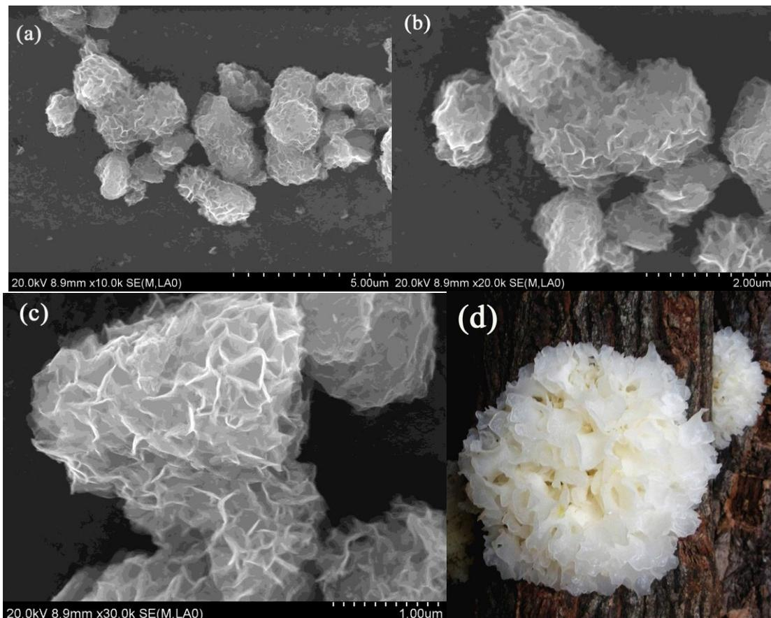
**Figure 1.** (a-c) SEM images of the tremella-like indium silver sulfide samples at different magnifications; (d) An image of native tremella
