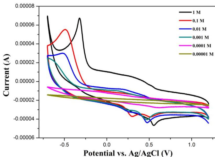
**Figure 6.** Effect of the H<sub>2</sub>SO<sub>4</sub> concentration on the CV behaviors of the TLISS/GCE with 2.84×10<sup>-4</sup> M 4-NP
