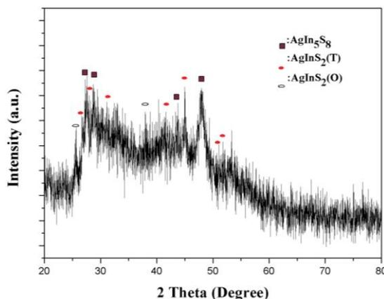
**Figure 2.** XRD pattern of the indium silver sulfide sample prepared by the co-precipitation method
