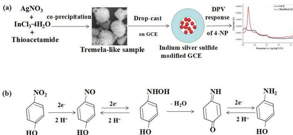
**Scheme 1.** (a) The illustration of indium silver sulfide sensing 4-NP by an electrochemical strategy; (b) The scheme of electron transfer in the detection of 4-NP.
