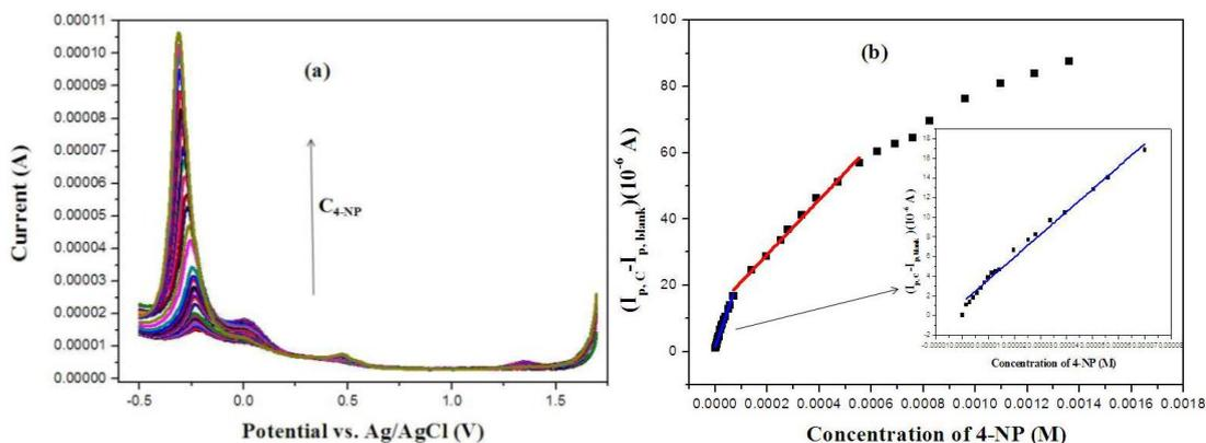
**Figure 7.** (a) DPV curves of the TLISS/GCE at different 4-NP concentrations in 1 M H<sub>2</sub>SO<sub>4</sub>; and (b) the corresponding calibration curves of 4-NP detection
