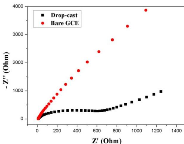
**Figure 5.** Nyquist plots of  $2.84 \times 10^{-4}$  M 4-NP in 1 M  $H_2SO_4$  for the bare GCE and TLISS/GCE, the frequency range: 10 kHz to 1 Hz; amplitude: 5 mV; and initial potential: 0.52 V
