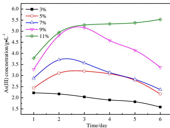
**Figure 2.** The As(III) concentration in the solution at different slurry densities in the first bio-oxidation process.
