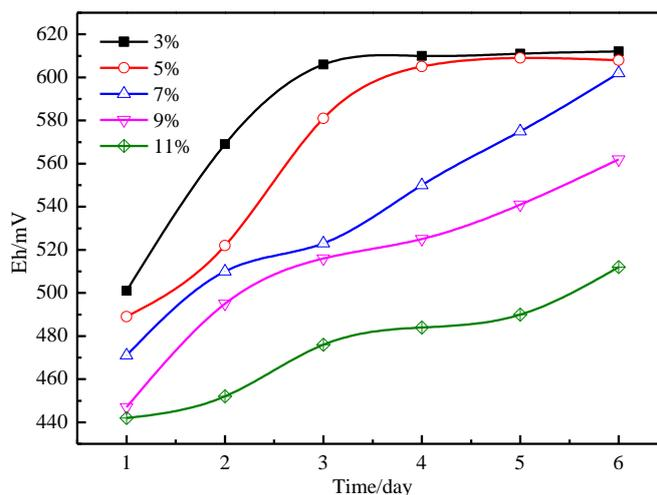
**Figure 1.** The redox potential of the solution at a different slurry density in the first-step bio-oxidation process.
