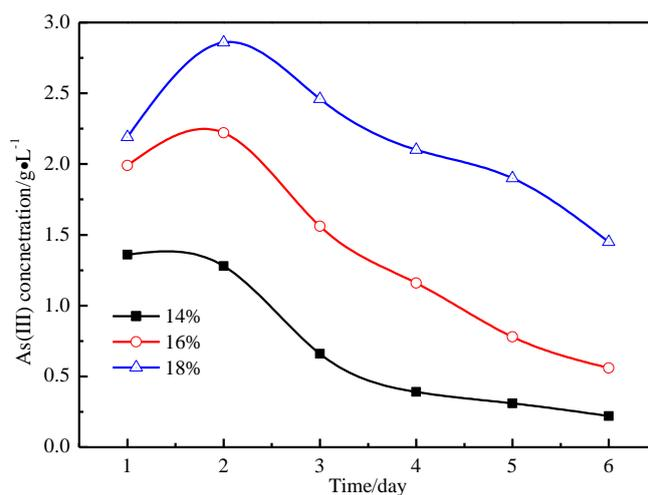
**Figure 5.** The As(III) concentration in the solution at different slurry densities in the second-step bio-oxidation process.
