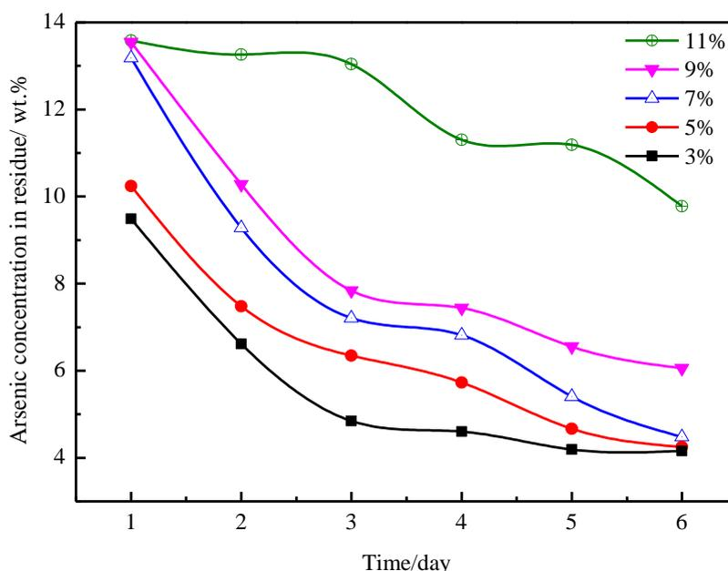
**Figure 3.** Arsenic content in the bioleaching residue after one-step bio-oxidation.
