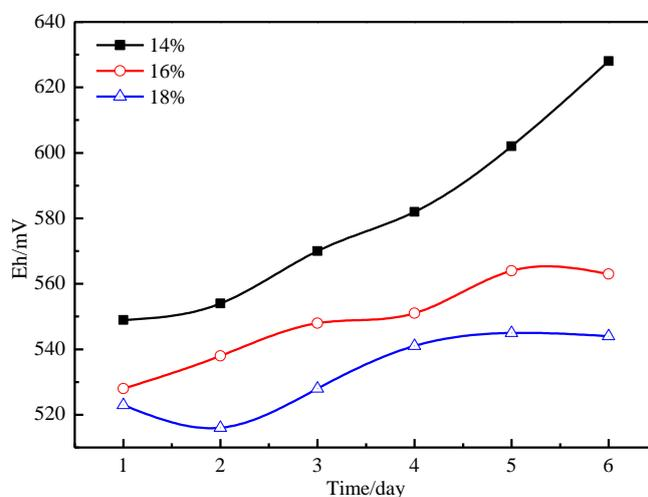
**Figure 4.** The redox potential of the solution at different slurry density in second-step bio-oxidation process.
