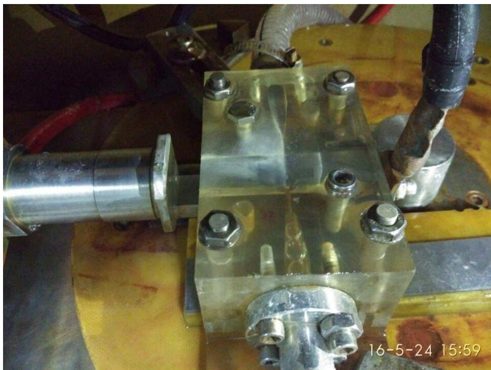
Figure 5. Test platform for side-flow electrochemical machining
