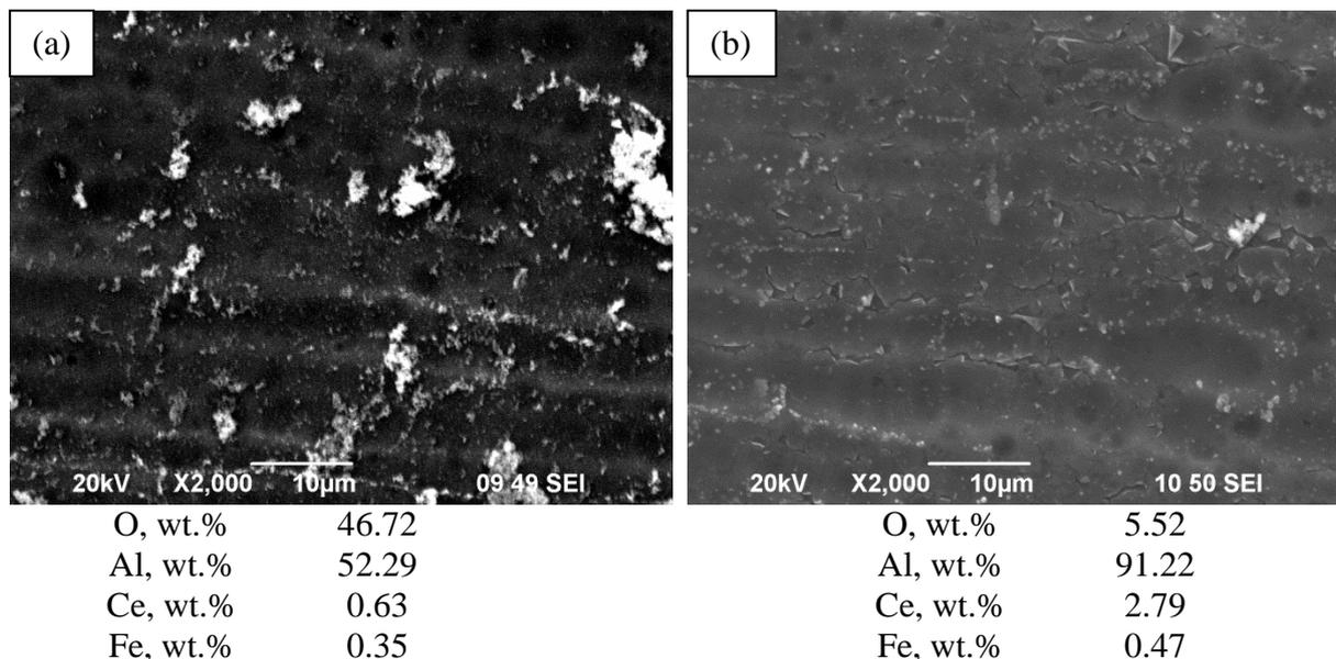
**Figure 2.** SEM micrographs and EDS data on the surface of the systems  $CeO_x/CeCl_3/Al_{NaOH}$  and  $CeO_x/CeCl_3/Al_{NaOH/HNO_3}$  obtained after: (a) pre-treatment of Al substrate in 1.5M NaOH; (b) pretreatment of Al substrate in 1.5M NaOH and 5M  $HNO_3$ .
