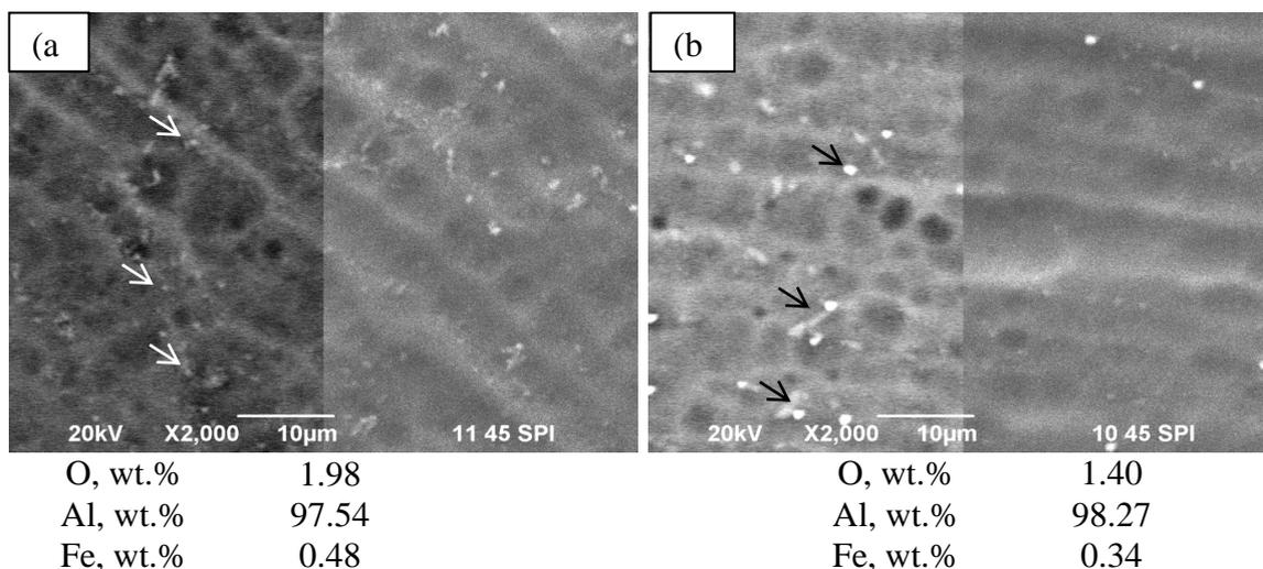
**Figure 1.** SEM micrograph of the surface of Al substrate (a) after pre-treatment in 1.5M NaOH; (b) after pre-treatment in 1.5M NaOH and in 5M  $\text{HNO}_3$ .
