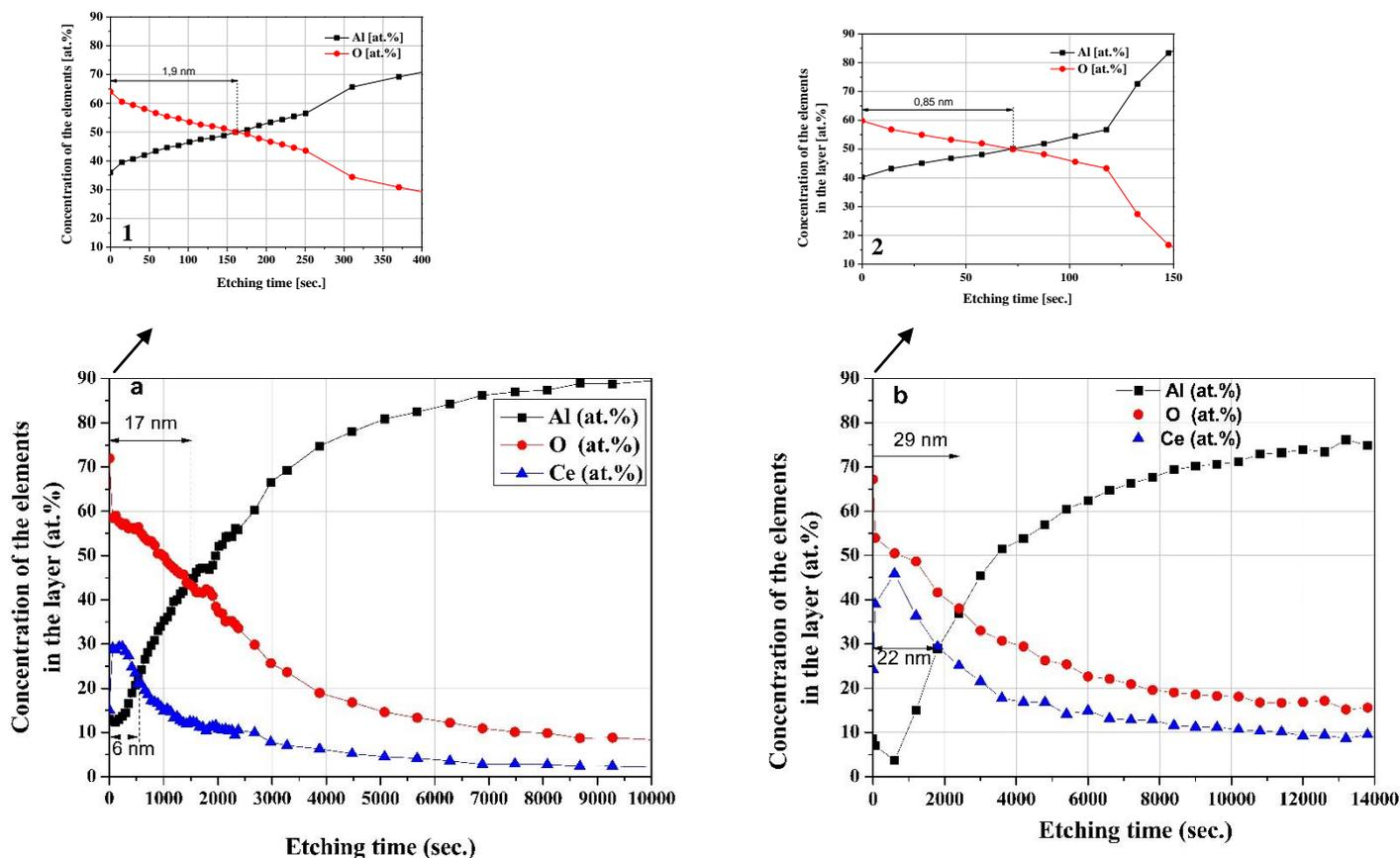
**Figure 4.** Depth profiles, displaying the change in the ratio between the elements Ce, Al and in the conversion layers (deposited from solution, containing only  $Ce^{3+}$  ions) on: (a)  $CeOx_{CeCl3}/Al_{NaOH}$  sample and (b)  $CeOx_{CeCl3}/Al_{NaOH/HNO3}$  sample. Depth profiles (inserts 1 and 2) show the change in the ratio between the elements Al and O in the surface layers formed on the Al substrate, after its pre-treatment in: 1 - 1.5M NaOH and 2 - 1.5M NaOH and 5M  $HNO_3$ .
