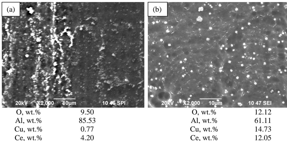
**Figure 3.** SEM micrograph and EDS data on the surface of the systems  $CeO_x/CeCl_3+CuCl_2/Al_{NaOH}$  and  $CeO_x/CeCl_3+CuCl_2/Al_{NaOH/HNO_3}$  obtained after: (a) pre-treatment of Al substrate in 1.5M NaOH; (b) pretreatment of Al substrate in 1.5M NaOH and 5M  $HNO_3$
