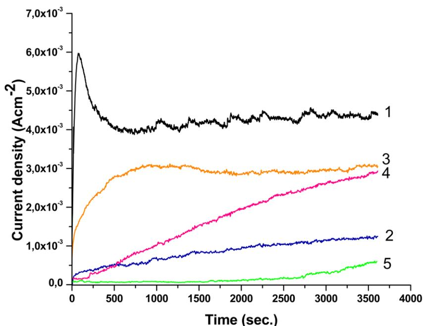
**Figure 8.** Chronoamperometric curves of the studied samples: 1 –  $\text{Al}/\text{Al}_2\text{O}_3$  native; 2 –  $\text{CeOx}_{\text{CeCl}_3}/\text{Al}_{\text{NaOH}}$ ; 3 –  $\text{CeOx}_{\text{CeCl}_3}/\text{Al}_{\text{NaOH}/\text{HNO}_3}$ ; 4 –  $\text{CeOx}_{\text{CeCl}_3+\text{CuCl}_2}/\text{Al}_{\text{NaOH}}$ ; 5 –  $\text{CeOx}_{\text{CeCl}_3+\text{CuCl}_2}/\text{Al}_{\text{NaOH}/\text{HNO}_3}$  in 0,1M  $\text{NaCl}$  at the pitting potential of Al ( $-0.5$  V vs. SCE).
