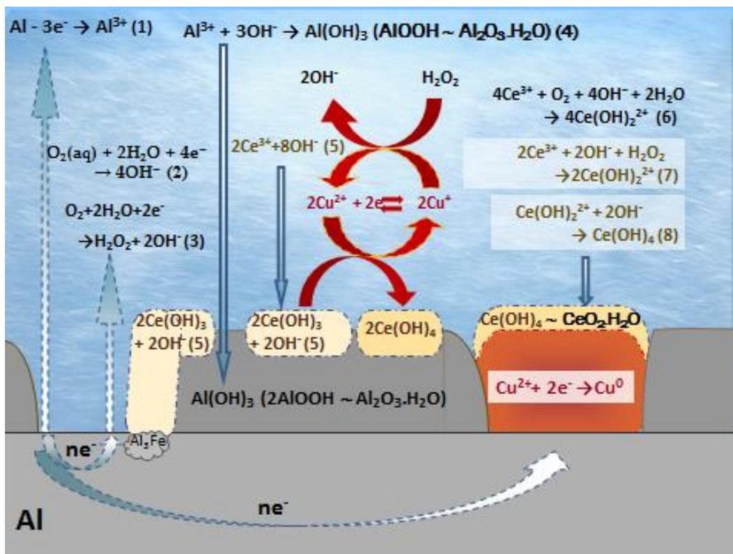
**Figure 6.** Scheme of the processes, occurring during deposition of cerium oxide(s) conversion layers on Al substrate from electrolytes, containing Ce<sup>3+</sup> and Cu<sup>2+</sup> ions.
