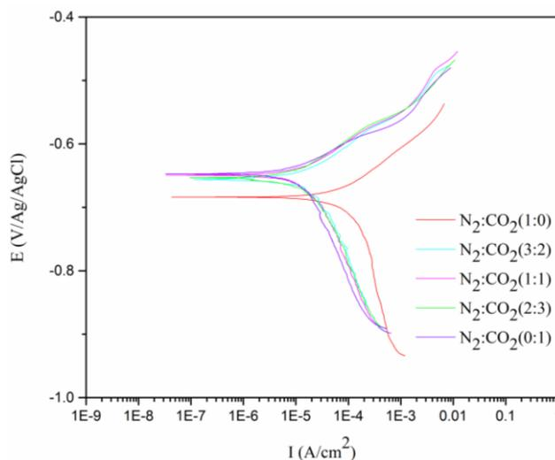
**Figure 14.** The effect of different partial pressures of CO<sub>2</sub> on the polarization curves of carbon steel in 0.5 mol% NH<sub>4</sub>Cl for exposure time up to 4 h at 55 °C.
