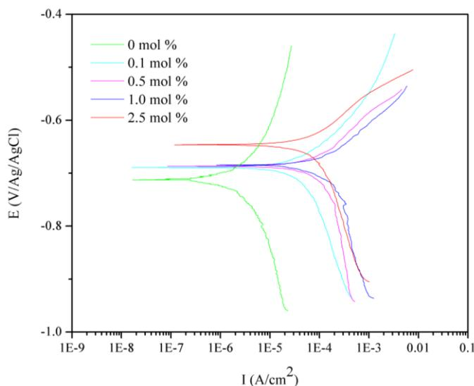
**Figure 7.** The effect of the different NH<sub>4</sub>Cl concentrations on the polarization curves of mild steel for an exposure time of 4 h at 55 °C.
