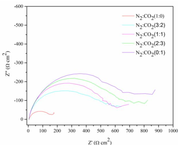
**Figure 15.** The effect of different partial pressures of CO<sub>2</sub> on the EIS of carbon steel in 0.5 mol% NH<sub>4</sub>Cl for exposure time up to 4 h at 55 °C.
