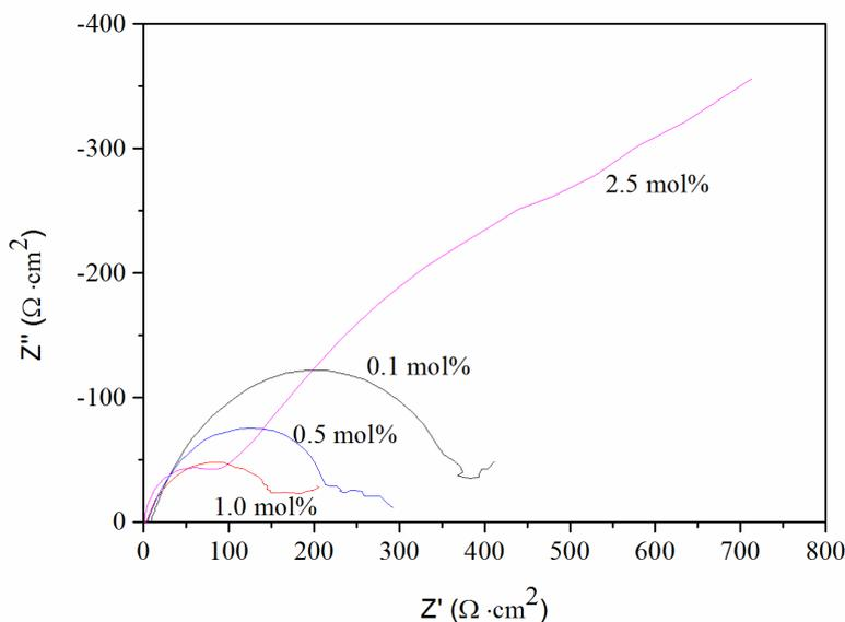
**Figure 8.** The effect of the different NH<sub>4</sub>Cl concentrations on the EIS of mild steel for an exposure time of 4 h at 55 °C.
