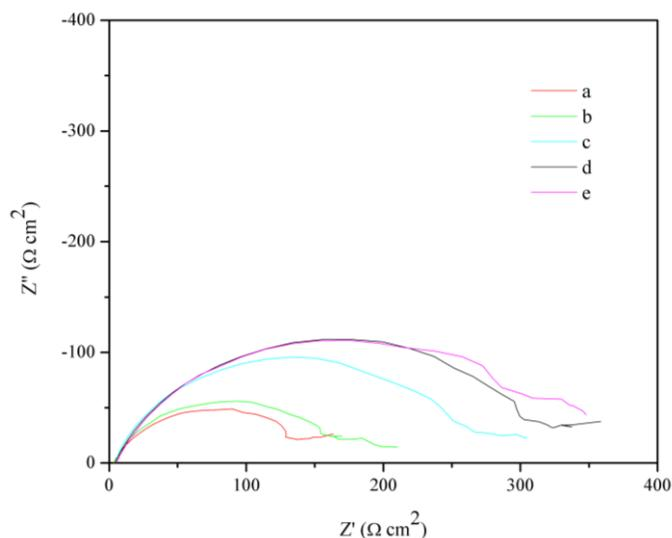
**Figure 2.** The effect of different surface roughnesses on the EIS of carbon steel in a 0.5 mol%  $\text{NH}_4\text{Cl}$  solution for an exposure time of 4 h at 25 °C: (a) surface ground to 600-grit finish; (b) surface ground to 1000-grit finish; (c) surface ground to 1500-grit finish; (d) surface ground to 2000-grit finish; (e) surface ground to 2000-grit finish and polished using  $\text{Al}_2\text{O}_3$  powder (0.001mm) impregnated polishing cloths.
