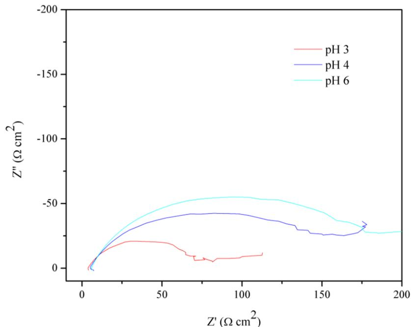
**Figure 13.** The effect of pH on the EIS of carbon steel in 0.5 mol% NH<sub>4</sub>Cl for an exposure time up to 4 h at 55 °C.
