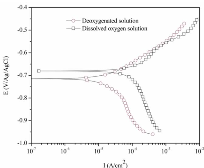
**Figure 4.** The effect of dissolved oxygen on the polarization curves of mild steel in a 0.5 mol% NH<sub>4</sub>Cl solution for an exposure time of 4 h at 25 °C.
