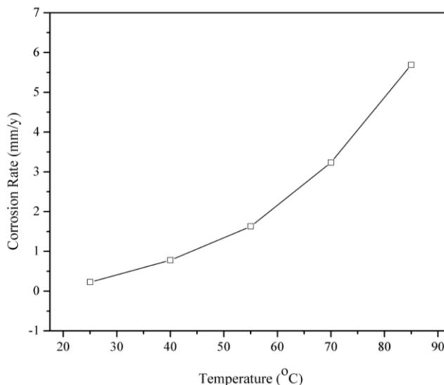
**Figure 6.** The effect of temperature on the corrosion rates of mild steel in 0.5 mol% NH<sub>4</sub>Cl solution for an exposure time of 4 h.
