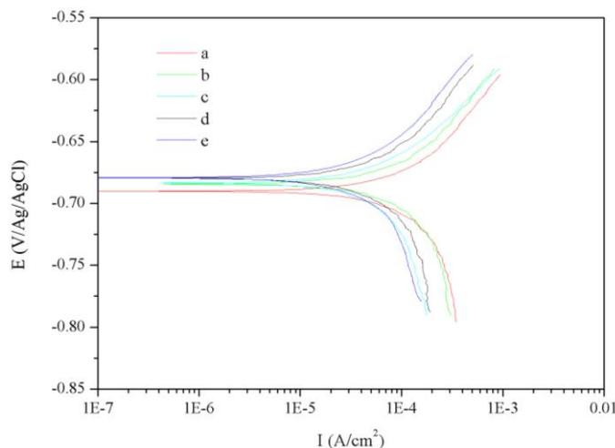
**Figure 1.** The effect of different surface roughnesses on the polarization curves of carbon steel in a 0.5 mol% NH<sub>4</sub>Cl solution for an exposure time of 4 h at 25 °C: (a) surface ground to 600-grit finish; (b) surface ground to 1000-grit finish; (c) surface ground to 1500-grit finish; (d) surface ground to 2000-grit finish; (e) surface ground to 2000-grit finish and polished using Al<sub>2</sub>O<sub>3</sub> powder (0.001mm) impregnated polishing cloths.
