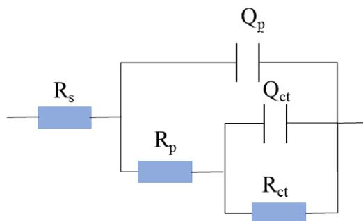
**Figure 3.** Electrical equivalent circuit used to fit the EIS curves of carbon steel in a 0.5 mol% NH<sub>4</sub>Cl solution for an exposure time of 4 h at 25 °C with different surface roughnesses.
