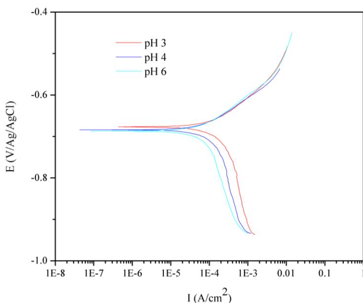
**Figure 12.** The effect of pH on the polarization curves of carbon steel in 0.5 mol%  $NH_4Cl$  for an exposure time up to 4 h at 55 °C.
