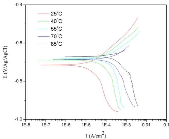
**Figure 5.** The effect of temperature on the polarization curves of mild steel in 0.5 mol% NH<sub>4</sub>Cl solution for an exposure time of 4 h.
