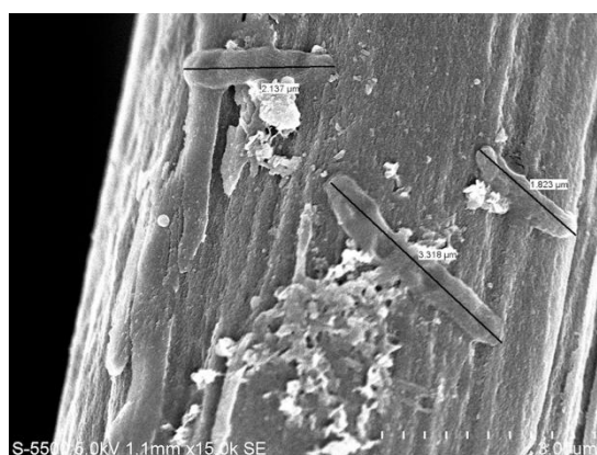
Figure 8. Micrograph obtained with the FESEM S5500 Hitachi. Bacteria enrichment during biofilm formation on the surface of the electrode treated during 36 h at 38 °C with a carbon source of 21 mM \text{NaCH}_3\text{COO} and an applied potential of 1.35 V (see E2 in table 3).
