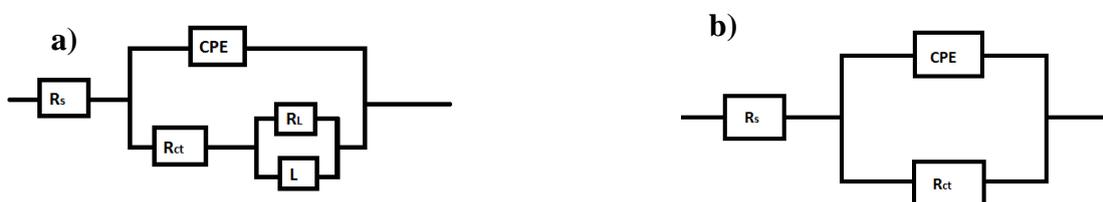
**Figure 7.** Equivalent circuits used for fitting data obtained by EIS from AISI 1018 Carbon steel in 0.5 M  $H_2SO_4$  at 25 °C. (a) Without and with 200 ppm of green inhibitor; (b) with 300 to 600 ppm of *P. persica* used as GCI.
