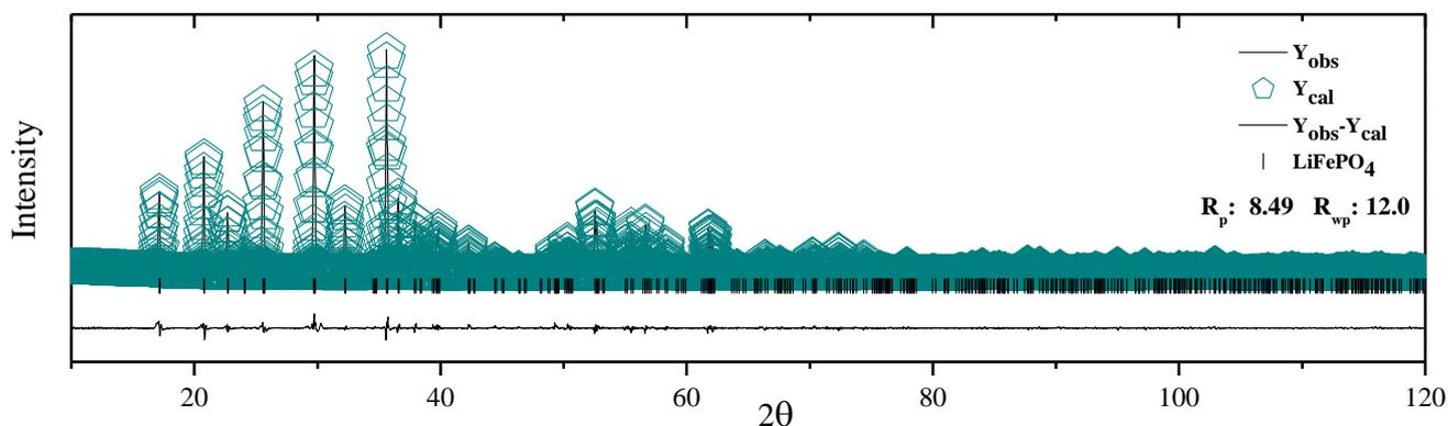
**Figure 2.** Rietveld refinement of pristine  $\text{LiFePO}_4$  after annealing.
