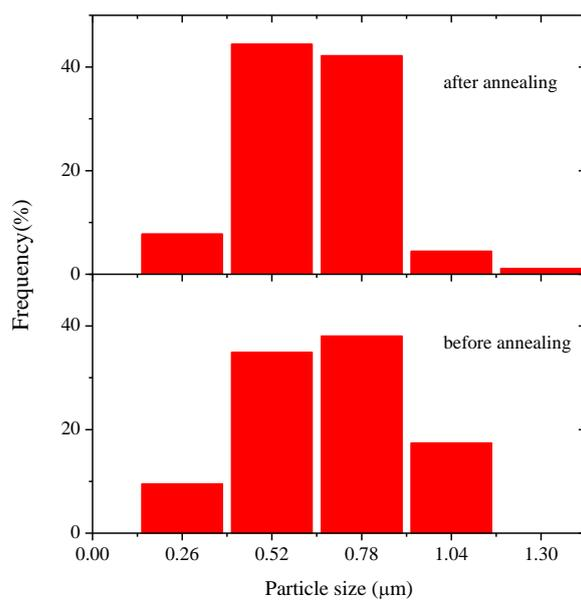
Figure 4. Comparison of particle size distribution of pristine LiFePO<sub>4</sub> before and after annealing.
