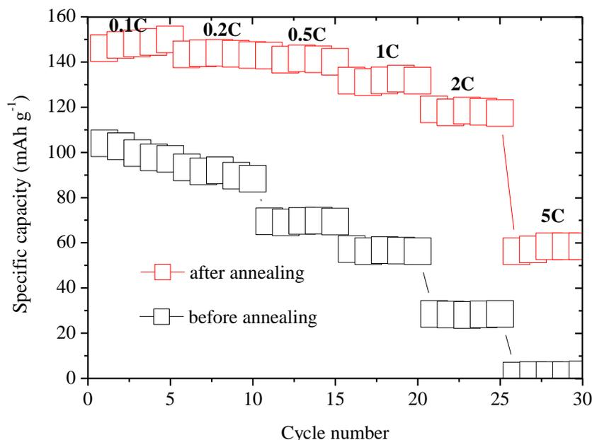
**Figure 7.** Cycle and Rate performance of pristine LiFePO<sub>4</sub> before and after annealing.
