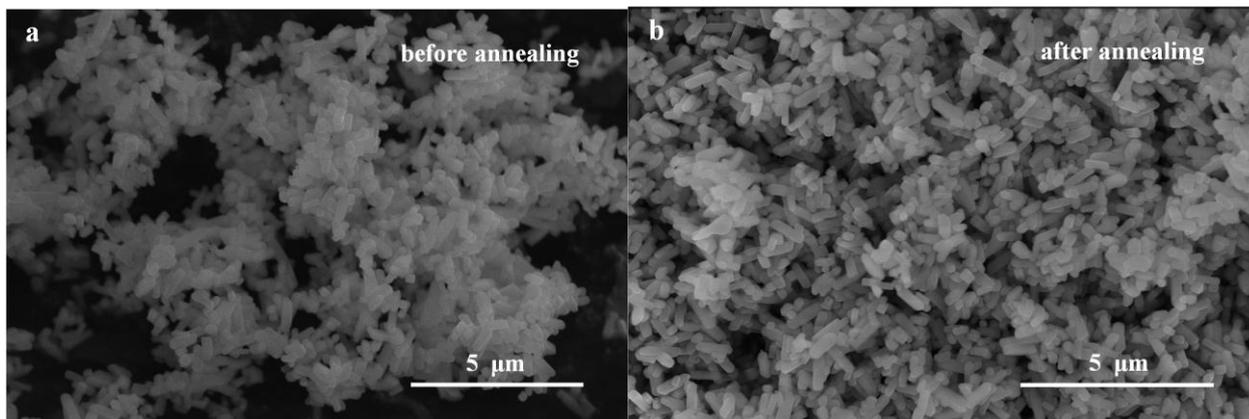
Figure 3. SEM images of pristine LiFePO<sub>4</sub> before and after annealing.
