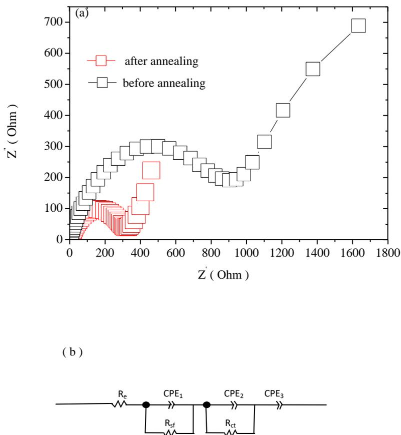
**Figure 8.** Impedance spectra of pristine  $\text{LiFePO}_4$  before and after annealing : (a) Nyquist plots; (b) equivalent circuit model. The frequency range and pulse amplitude applied were 100 kHz-100 mHz and 5 mV, respectively.
