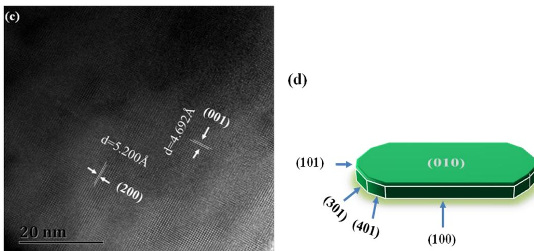
**Figure 5.** TEM image and the selected area electron diffraction (SAED) pattern of pristine  $\text{LiFePO}_4$  after annealing (a,b).  $\text{LiFePO}_4$  hexagonal nanorods have predominant (010) face exposure, and the side of nanorods is (100) plane. HRTEM and simulated morphology of  $\text{LiFePO}_4$  crystal (c,d).
