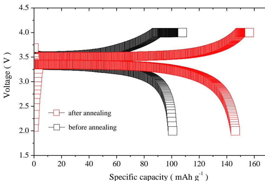
**Figure 6.** Comparison of initial charge-discharge curves of pristine  $\text{LiFePO}_4$  before and after annealing at 0.1C.
