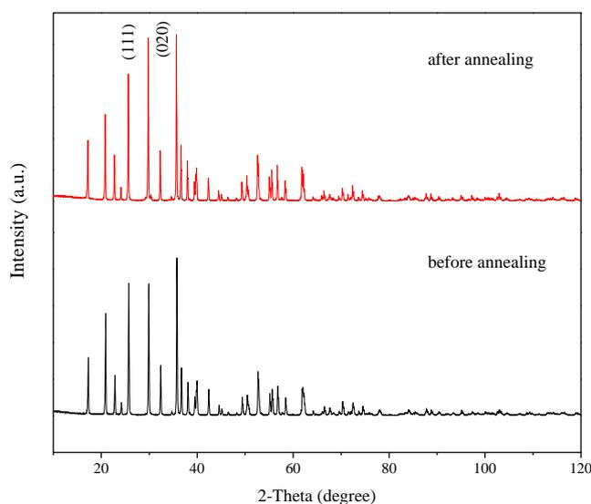
**Figure 1.** XRD pattern of pristine  $\text{LiFePO}_4$  before and after annealing.
