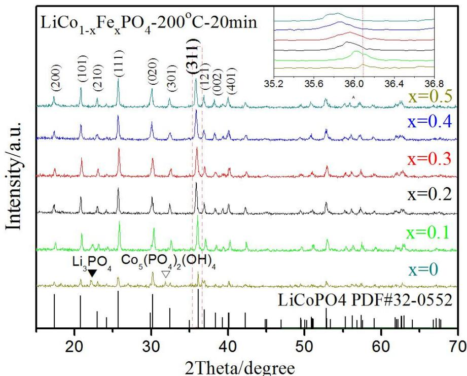
**Figure 1.** XRD patterns of the  $\text{LiCo}_{1-x}\text{Fe}_x\text{PO}_4/\text{C}$  ( $0 \leq x \leq 0.5$ ) samples. Inset image: Diffraction peaks of crystal face (311).
