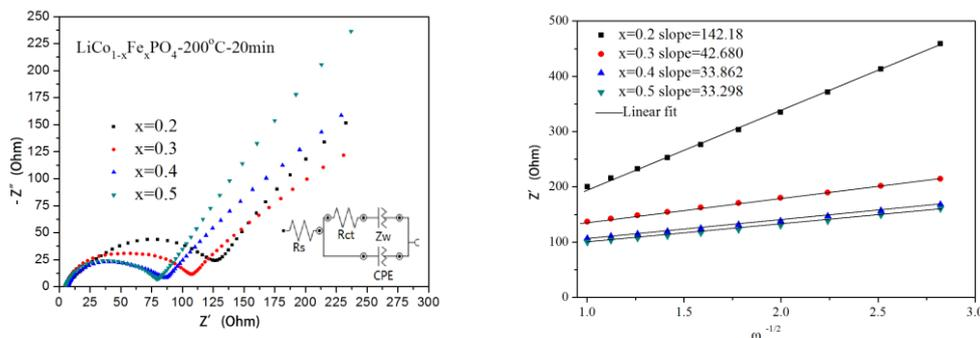
**Figure 5.** Profiles of electrochemical impedance spectroscopy (EIS). (a) Nyquist curve (b) linear fitting of  $Z' - \omega^{-1/2}$
