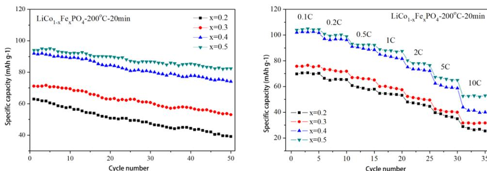
**Figure 4.** (a) Cycling performance of LiCo<sub>1-x</sub>Fe<sub>x</sub>PO<sub>4</sub>/C (0.2 ≤ x ≤ 0.5) at 0.5C, (b) rate performance of LiCo<sub>1-x</sub>Fe<sub>x</sub>PO<sub>4</sub>/C (0.2 ≤ x ≤ 0.5) samples at different current densities
