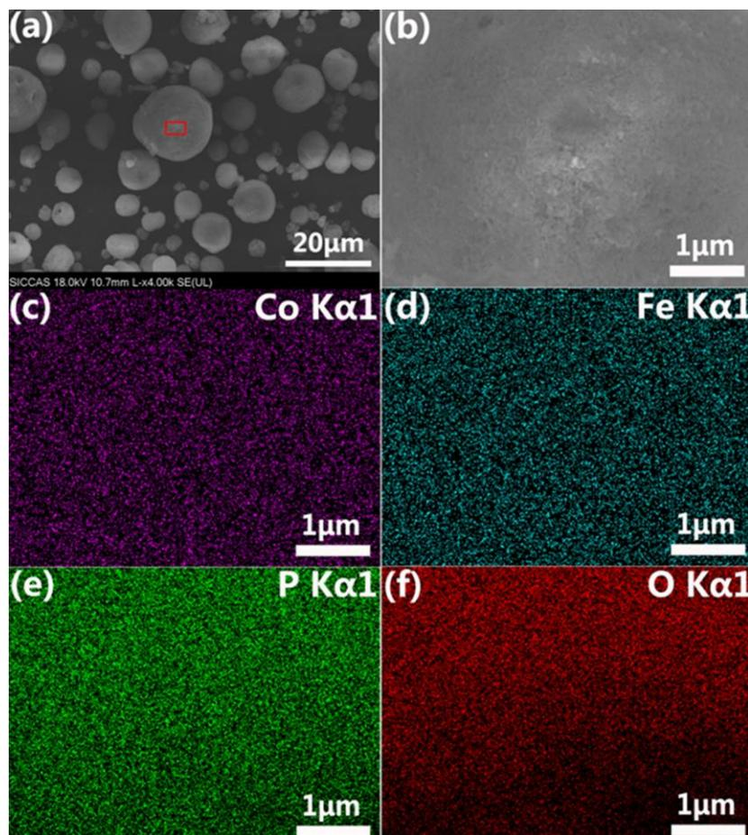
**Figure 2.** SEM images (a,b) and the elemental mappings of Co (c), Fe (d), P (e) and O (f) for the  $\text{LiCo}_{0.5}\text{Fe}_{0.5}\text{PO}_4/\text{C}$  sample
