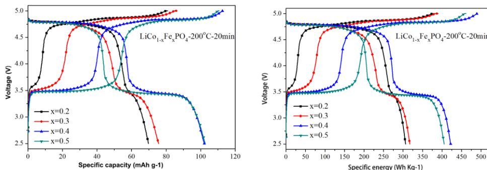
**Figure 3.** The first charge/discharge profiles of LiCo<sub>1-x</sub>Fe<sub>x</sub>PO<sub>4</sub>/C (x ≤ 0.5) at 0.1C (a) capacity-voltage (b) energy-voltage
