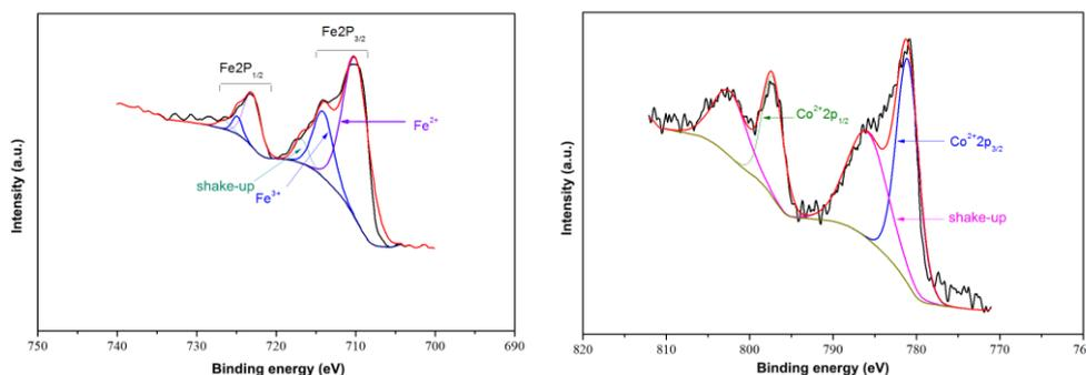
**Figure 6.** (a) Fe2p and (b) Co 2p XPS spectra of the  $LiCo_{0.5}Fe_{0.5}PO_4/C$
