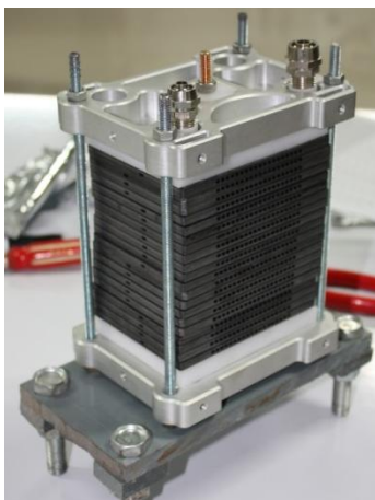
Figure 1. 10-cell stack on the lab bench
