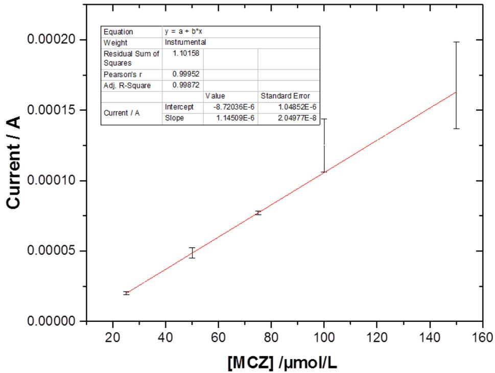
**Figure 5.** Calibration curve MCZ (25, 50, 75, 100 and 150 μmol/L) in BRBS at pH 7 using a PEDOT/MWCNT electrode.
