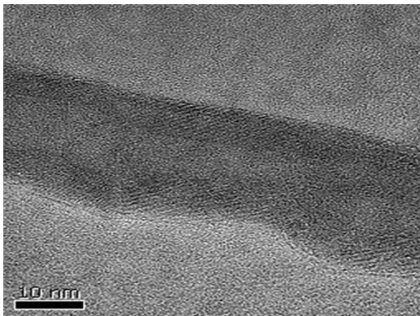
**Figure 1.** Transmission electron microscopy image of MWCNTs along with sodium dodecyl sulfate (SDS) as surfactant.
