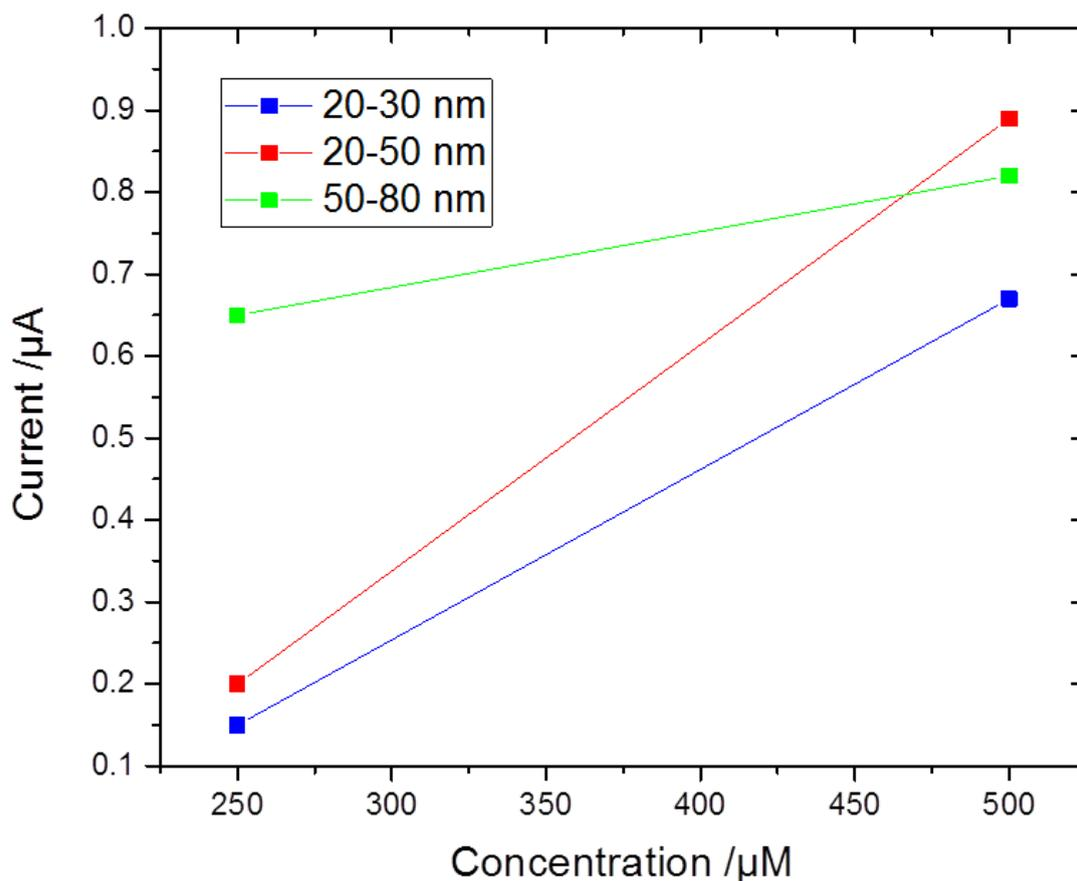
**Figure S1.** Current peaks vs concentration for polymerized electrodes with CNTs at 20-30 nm, 30-50 nm and 50-80 nm diameters in PEDOT.
