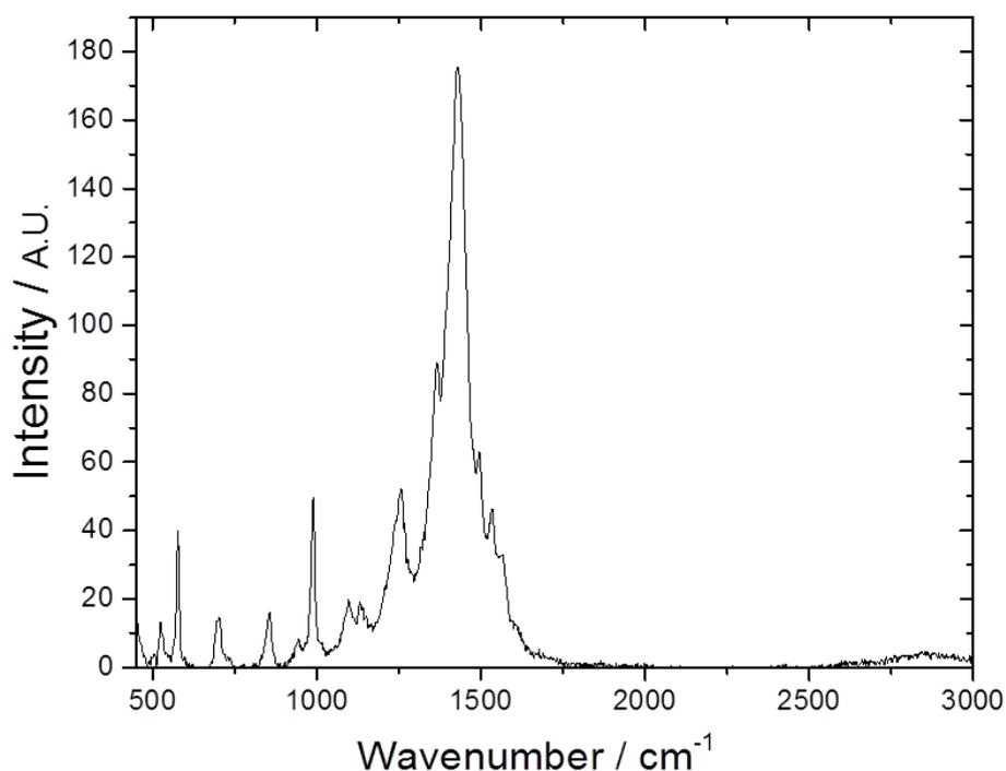
**Figure 2.** Raman spectra of MWCNTs electropolymerized in the PEDOT matrix.
