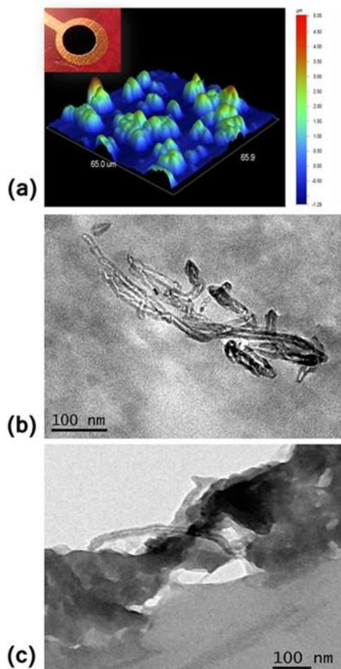
**Figure 3.** Coated electrode images: a) electrode surface roughness (inset: PEDOT/MWCNT-coated electrode), b) MWCNT aggregates inside the PEDOT layer and c) MWCNT anchored to the PEDOT layer.
