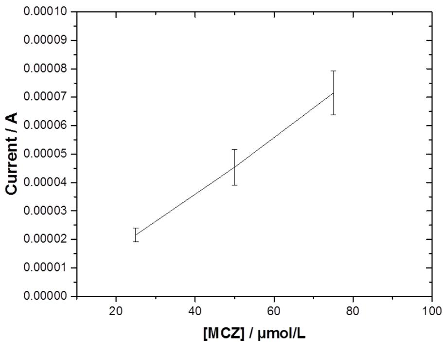
**Figure 6.** Calibration curve MCZ (25, 50 and 75 μmol/L) in BR buffer at pH 7 using a PEDOT/MWCNT electrode.
