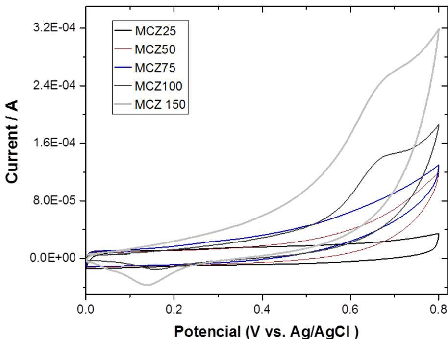
**Figure 4.** Voltammograms obtained for different MCZ concentrations of 0, 25, 50, 75, 100, 150, 200 and 250  $\mu\text{mol/L}$  in BRBS at pH 7 using the PEDOT/MWCNT electrode.
