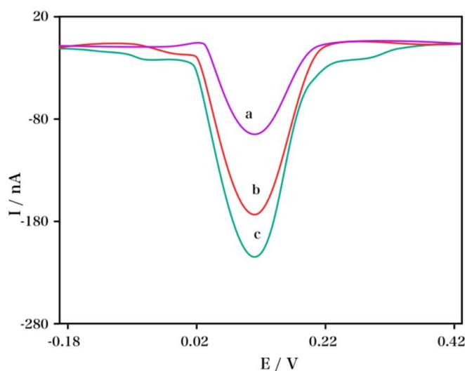
**Figure 2.** DPV curves for the  $\beta\text{-CD}$  accumulated on the ds-DNA/SAM surface synthesized via different hybridization strategies: (a) the drop method, (b) the preheated solution method and (c) the solution hybridization method.
