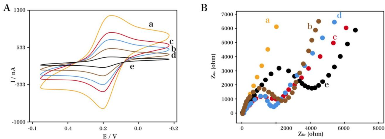
**Figure 5.** (A) CV recorded the coated electrode in 1.0 mM of  $K_3[Fe(CN)_6]$  solution after each electrode modification procedure: (a) bare AuE, (b) ss-DNA-coated AuE, (c) MCH/ss-DNA-coated AuE, (d) mismatched target DNA, and (e) target DNA. (B) The Nyquist plot of these electrodes in 5.0 mM of  $K_3[Fe(CN)_6]/K_4[Fe(CN)_6]$  that contained 1.0 M of KCl: (a) bare AuE, (b) ss-DNA-coated AuE, (c) MCH/ss-DNA-coated AuE, (d) mismatched target DNA, and (e) target DNA.
