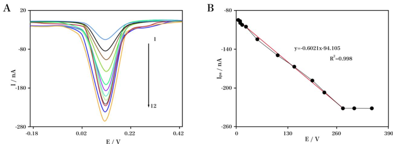
**Figure 6.** (A) DPV curves for the accumulated  $\beta$ -CD on the hybridized ss-DNA-coated AuE with the complementary (target) DNA at different concentrations in 0.1 M of PBS (pH 7.0). (B) Inset: the variation in the accumulated current response on ds-DNA-coated AuE and ss-DNA/SAM vs. the target DNA concentration during hybridization.
