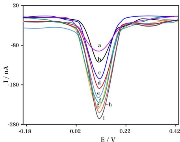
**Figure 3.** (A) DPV curves for the  $\beta$ -CD accumulated on the ds-DNA/SAM surface synthesized in the presence of  $\beta$ -CD at different concentrations over a range of 0.015-0.135 mM, as shown in (a) to (i).
