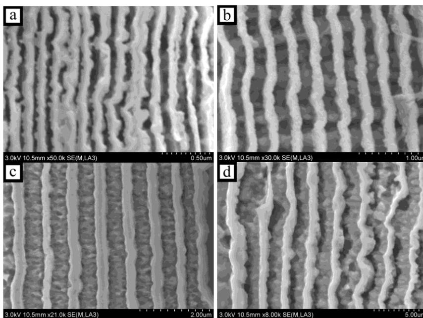
**Figure 2.** Cross-sectional micrographs of the multilayer films prepared at different switching ratios: (a) 10/10, (b) 30/30, (c) 50/50, (d) 100/100
