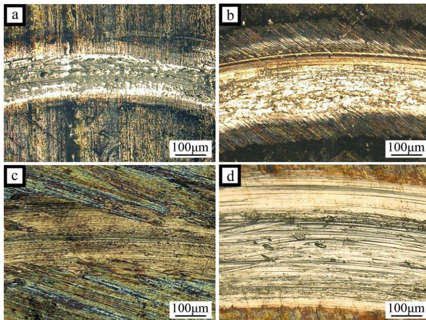
**Figure 7.** Worn surface morphologies of the multilayer films prepared at different switching ratios: (a) 1/1, (b) 3/3, (c) 5/5, (d) 10/10
