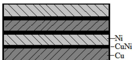
**Figure 5.** Schematic diagram of the three layer structure of Cu-Ni multilayer film
