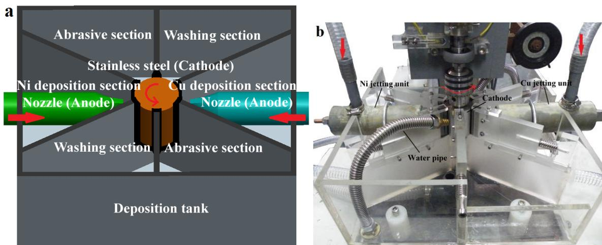
**Figure 1.** Experimental Platform: (a) Schematic diagram, (b) Physical picture
