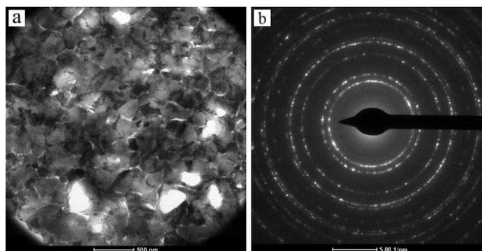
**Figure 4.** TEM field diagram of Cu-Ni multilayer film (a) and its corresponding electron diffraction pattern (b)
