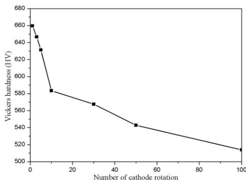
**Figure 6.** Microhardness of Cu-Ni multilayer films
