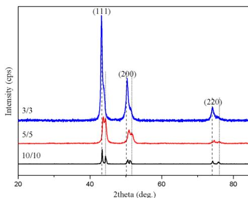
**Figure 3.** X-ray diffraction patterns of the multilayer films prepared at different switching ratios
