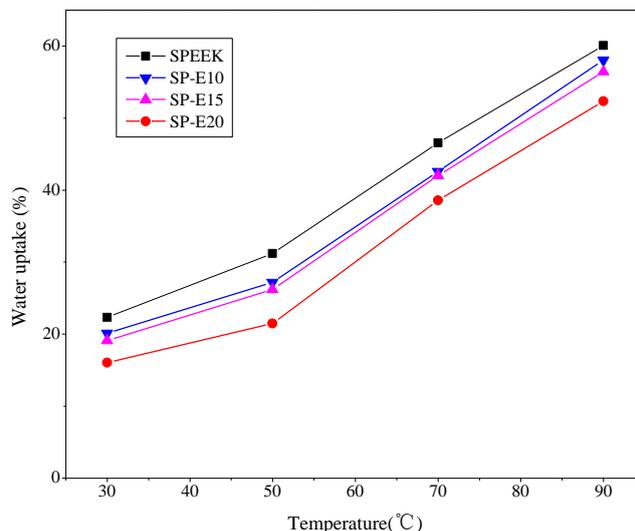
**Figure 6.** Water uptake of pure SPEEK membrane and SPEEK/epoxy semi-interpenetrating network membranes vs temperature
