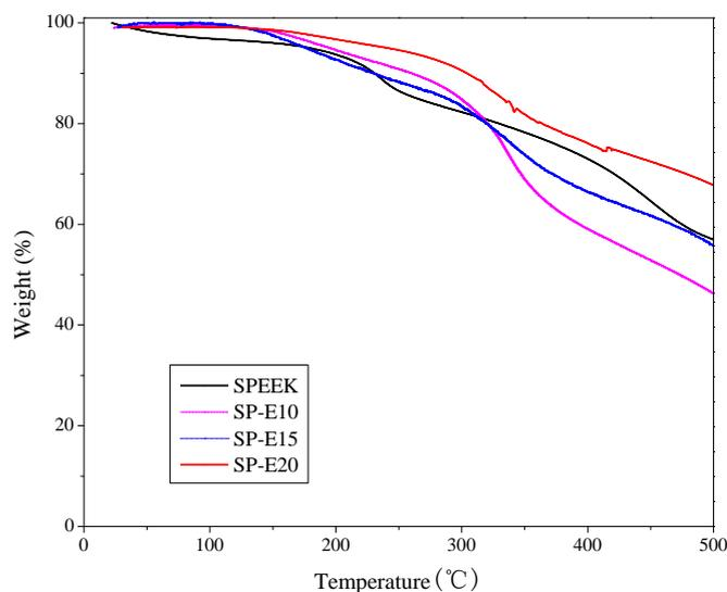
**Figure 3.** TG curves of SPEEK/epoxy semi-interpenetrating network membranes with different epoxy contents
