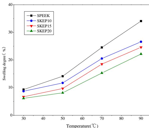
**Figure 7.** Swelling degree of SPEEK/epoxy semi-interpenetrating network membranes vs temperature
