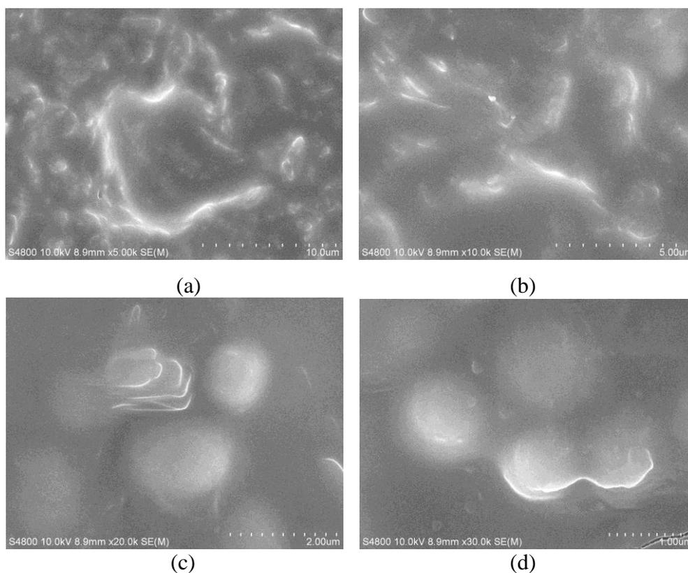
**Figure 2.** Morphology of SP-E15 SPEEK/epoxy semi-interpenetrating network membrane in different magnification: x5000, x10000, x20000 and x30000
