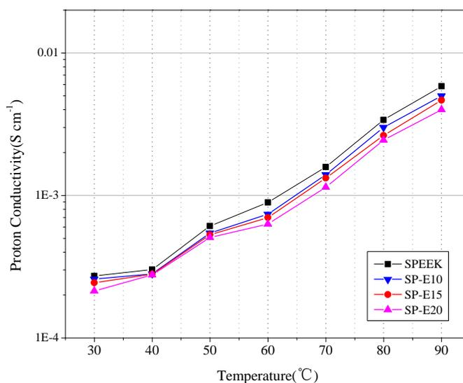
**Figure 4.** Proton conductivity of SPEEK/epoxy semi-interpenetrating network membranes vs temperature
