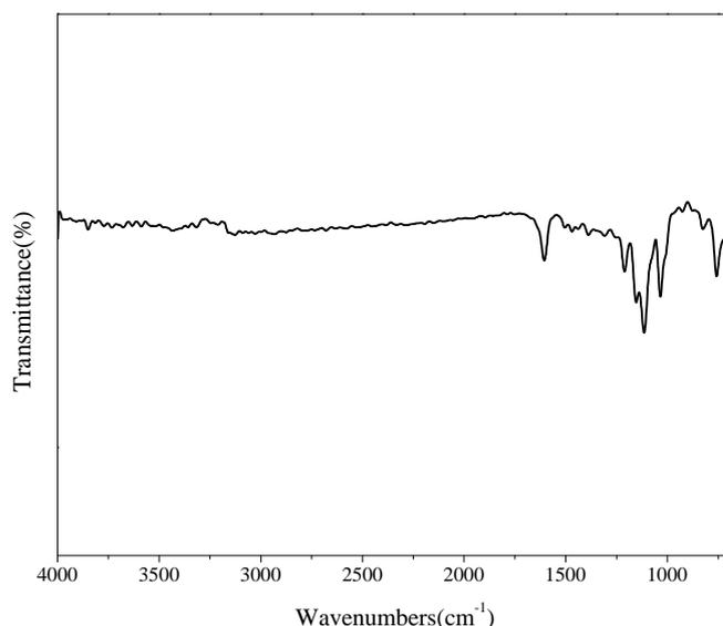
**Figure 1.** The FTIR spectrum of SPEEK/epoxy semi-interpenetrating network membrane
