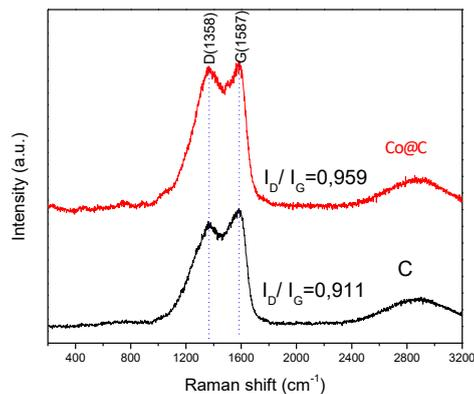
**Figure 2.** Raman spectra of Co@C and C
