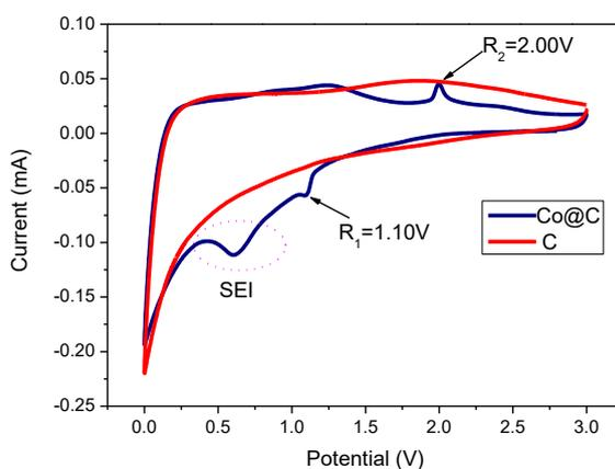
**Figure 5.** CV profiles of C and Co@C at scan rate of 0.1 mV.s<sup>-1</sup>
