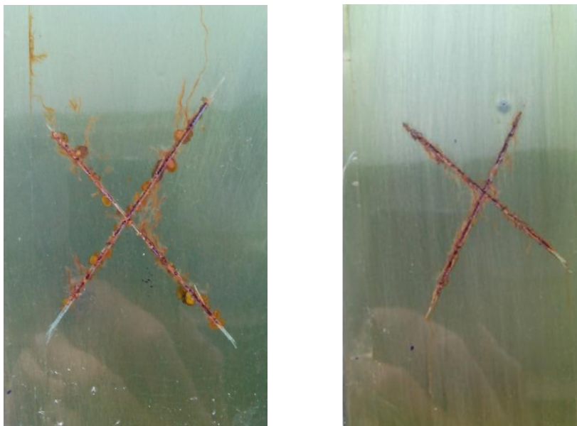
Figure 8. Corrosion morphology of coating after 90 hours of neutral salt spraying: (a) without; (b) with talcum powder loaded with 5 g/L sodium tungstate.
