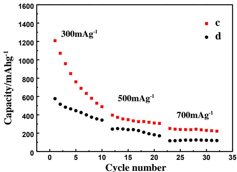
**Figure 6.** Rate capabilities of the produced half-cells at 300, 500, 700 mA g<sup>-1</sup>. Curves c and d were for the half-cells constructed by sample c and d.
