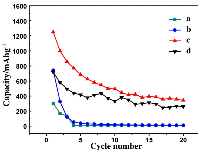
**Figure 5.** Cycling performances of all produced half-cells at 100 mA g<sup>-1</sup>. Curves a, b, c and d were for the half-cells constructed by sample a, b, c and d.
