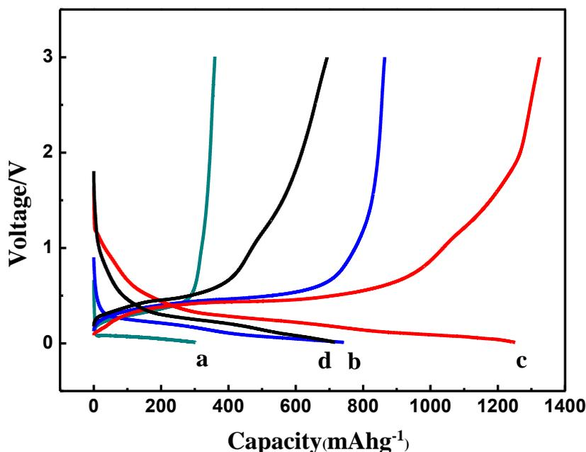
**Figure 4.** The initial galvanostatic charge-discharge plots in the potential range from 0V to 3V at  $100 \text{ mA g}^{-1}$ . Plots a, b, c and d were for the half-cells assembled by sample a, b, c and d.
