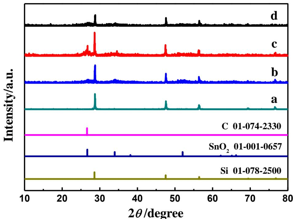
**Figure 1.** XRD patterns for the synthesized samples including the standard XRD patterns of Si, SnO<sub>2</sub> and C. Pattern a, b, c, and d is for sample a, b, c and d.
