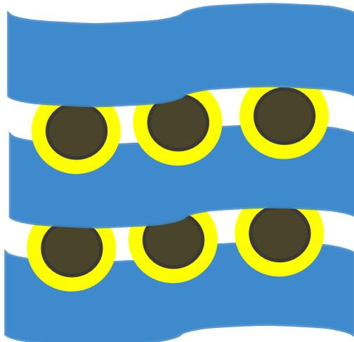
**Figure 10.** The structure schematic diagram for sample c, in which the black particle stood for the elementary Si, the yellow layer represented the formed  $\text{SnO}_2$ , and the blue ribbon corresponded to graphene.
