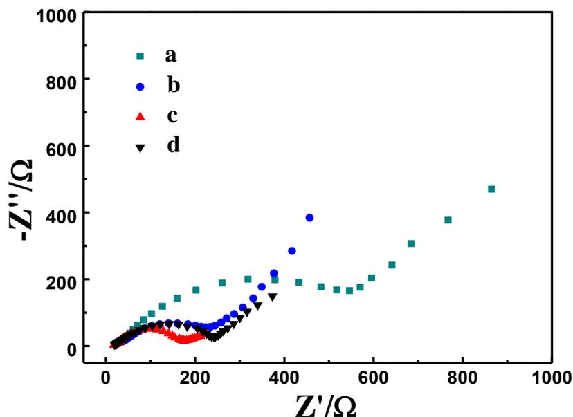
**Figure 8.** Nyquist plots of all prepared half-cells. Curves a, b, c and d were for the half-cells assembled by sample a, b, c and d.
