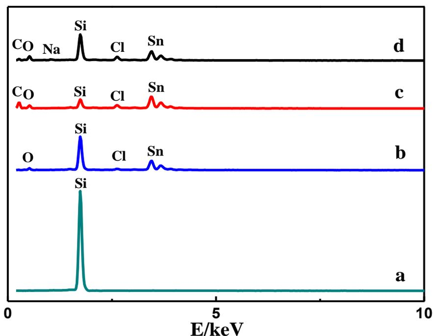
**Figure 2.** EDS spectra for all the produced samples. Curves a, b, c and d are for sample a, b, c and d.
