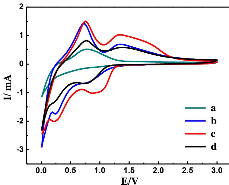
**Figure 7.** Cyclic voltammograms (CVs) of all the half-cells which were measured at 1 mV s<sup>-1</sup>. Curve a, b, c and d were for the half-cells fabricated by sample a, b, c and d.
