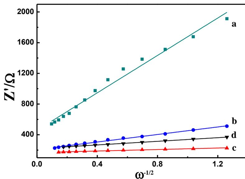
**Figure 9.** The typical curves describing the relationship between  $Z''$  and  $\omega^{-1/2}$ . Curve a, b, c and d were for the half-cells prepared by sample a, b, c and d.
