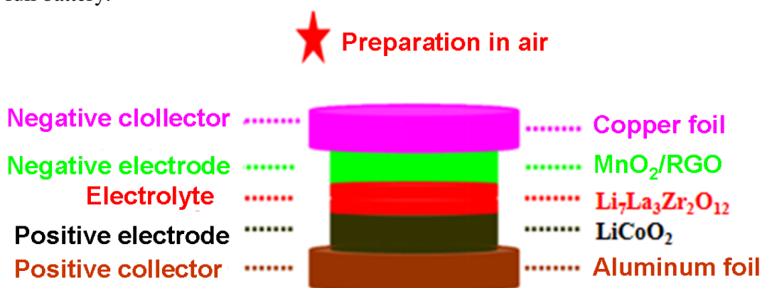
Figure 1. All solid state lithium ion batteries.
