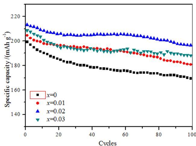
**Figure 4.** Cycle performances of  $\text{Li}_{1.20}[\text{Mn}_{0.54}\text{Ni}_{0.13}\text{Co}_{0.13}]\text{O}_2$  ( $x = 0, 0.01, 0.02, 0.03$ ).
