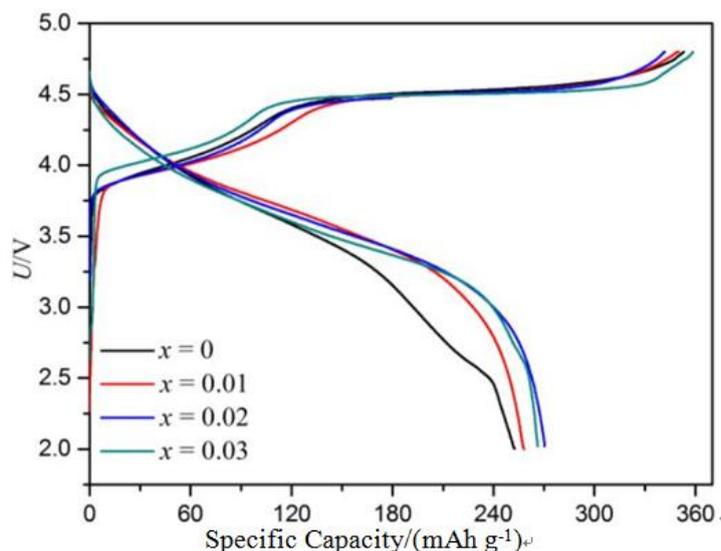
**Figure 3.** Initial charge and discharge curves of  $\text{Li}_{1.20}[\text{Mn}_{0.54}\text{Ni}_{0.13}\text{Co}_{0.13}]\text{O}_2$  ( $x = 0, 0.01, 0.02, 0.03$ )
