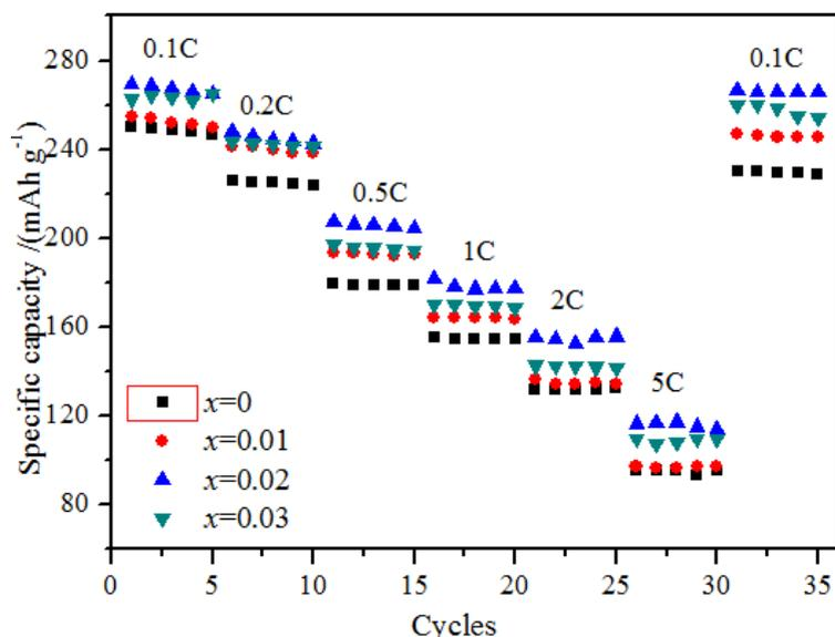
**Figure 5.** Rate capacities of  $\text{Li}_{1.20}[\text{Mn}_{0.54}\text{Ni}_{0.13}\text{Co}_{0.13}]\text{O}_2$  ( $x = 0, 0.01, 0.02, 0.03$ ).
