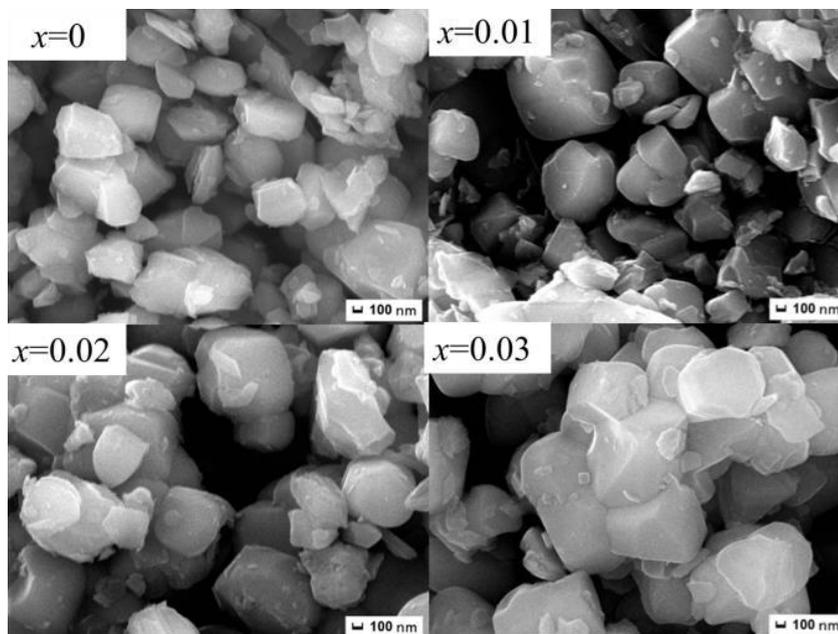
**Figure 2.** SEM images of  $\text{Li}_{1.20}[\text{Mn}_{0.54-x}\text{Ni}_{0.13}\text{Co}_{0.13}\text{Er}_x]\text{O}_2$  ( $x = 0, 0.01, 0.02, 0.03$ ).
