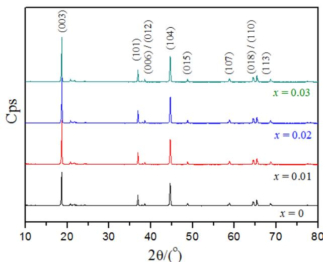
**Figure 1.** XRD spectra of  $\text{Li}_{1.20}[\text{Mn}_{0.54-x}\text{Ni}_{0.13}\text{Co}_{0.13}\text{Er}_x]\text{O}_2$  ( $x = 0, 0.01, 0.02, 0.03$ ).
