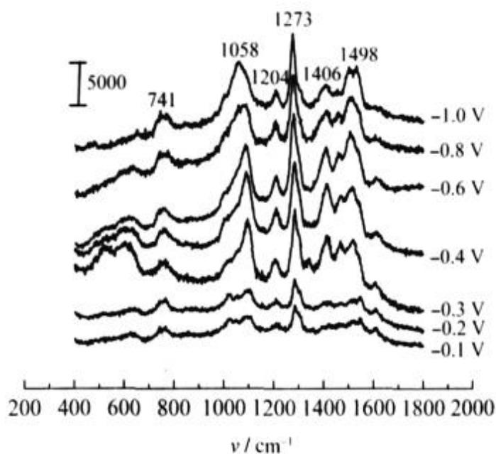
**Figure 8.** SERS spectra of  $0.24 \text{ mmol}\cdot\text{L}^{-1}$  ATA on copper at different potentials
