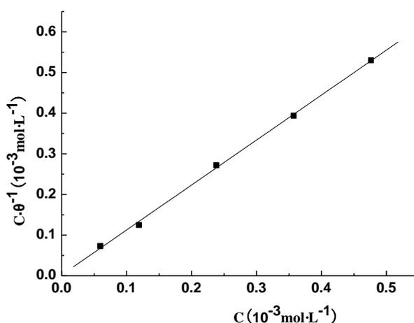
**Figure 5.** Curve fitting of the corrosion data for copper electrode according to Langmuir thermodynamic kinetic
