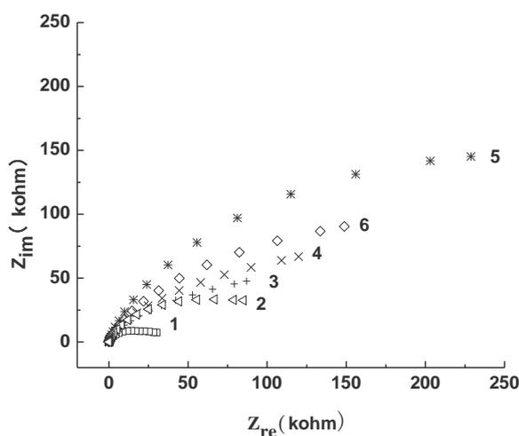
**Figure 3.** Nyquist plots for copper in borax buffer solution (pH=9.2) with different concentrations of ATA.  $C_{ATA}/(\text{mg}\cdot\text{L}^{-1})$ : (1) 0, (2) 5, (3) 10, (4) 20, (5)30, (6)40
