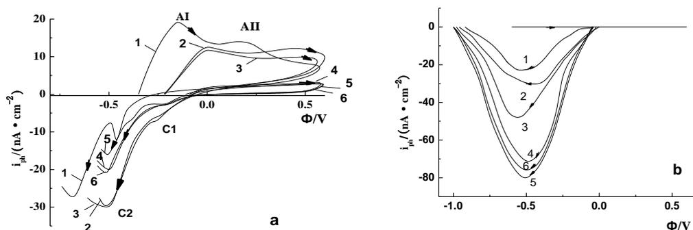
**Figure 2.**  $i$ - $\phi$  (a) and  $i_{\text{ph}}$ - $\phi$ (b) curves for copper electrode in borax buffer solution with different concentrations of ATA. Scan rate:  $1 \text{ mV/s}$ ; modulation frequency:  $39 \text{ Hz}$ ; irradiation wavelength:  $420 \text{ nm}$ ;  $C_{\text{ATA}}/(\text{mg}\cdot\text{L}^{-1})$ : (1) 0, (2) 5, (3) 10, (4) 20, (5)30, (6)40
