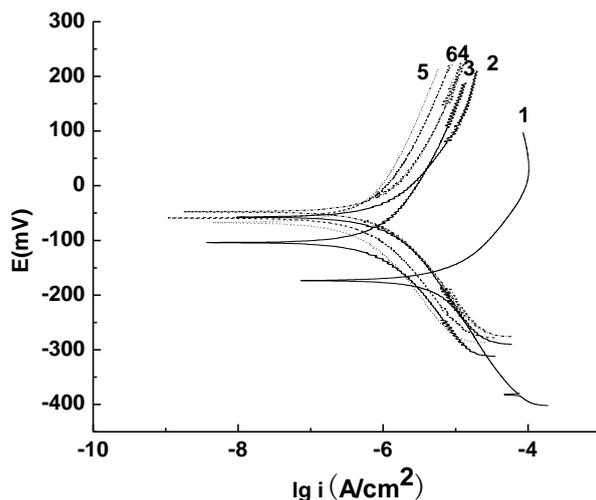
**Figure 4.** Potentiodynamic polarization curve plots for copper in borax buffer solution (pH=9.2) with different concentrations of ATA.  $C_{ATA}/(\text{mg}\cdot\text{L}^{-1})$ : (1) 0, (2) 5, (3) 10, (4) 20, (5)30, (6)40
