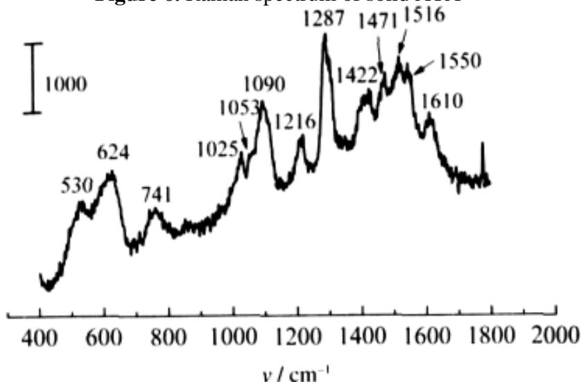
Figure 7. SERS spectrum of ATA adsorbed onto copper at open circuit potential (-0.21 V)
