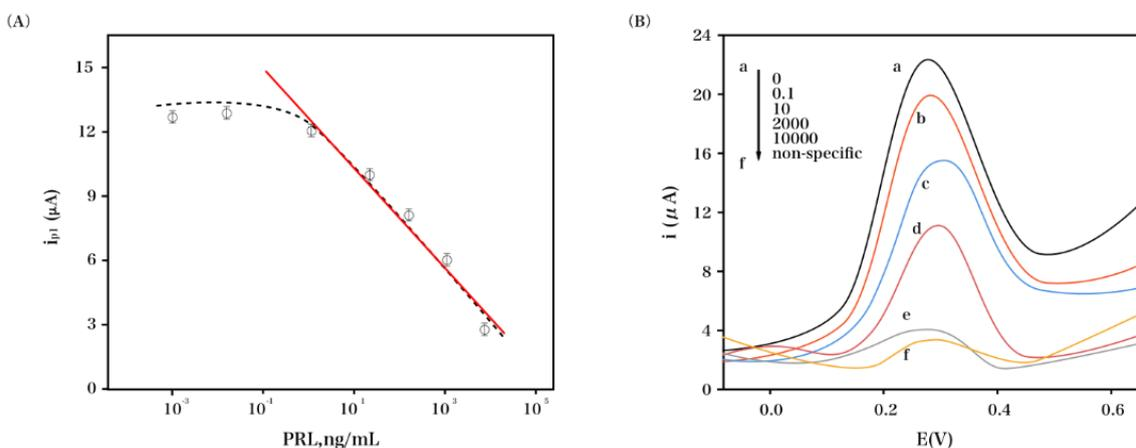
**Figure 2.** (A) Calibration curve for PRL in semilogarithmic form using the AP-anti-PRL-PRL-pPPA/MWCNTs modified GCE. (B) DPV patterns obtained for varying concentrations of PRL (0 - 10,000 ng/mL).
