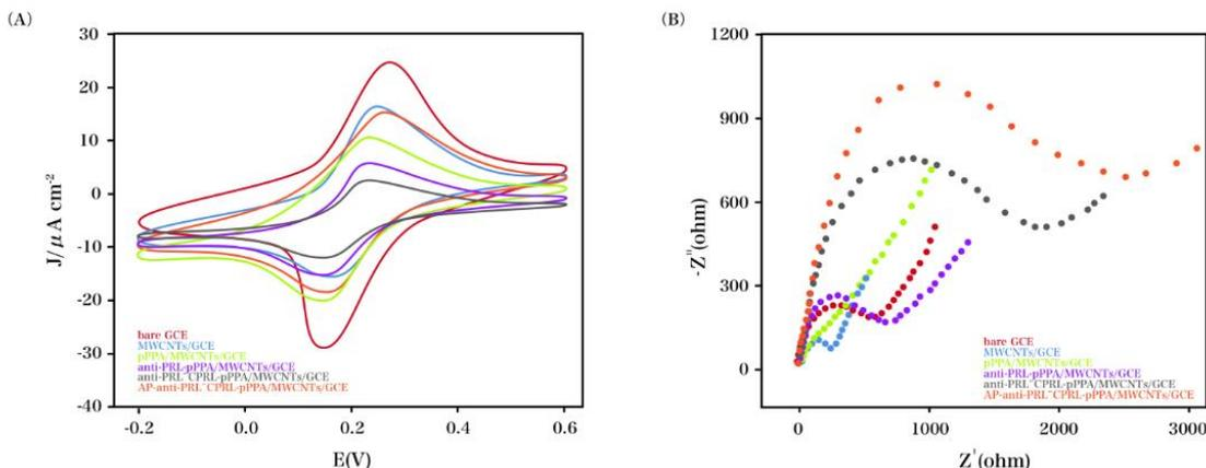
**Figure 1.** (A) CVs and (B) EIS spectra of each immobilization step in pH 7.4 PBS that contained  $[\text{Fe}(\text{CN})_6]^{3-/4-}$  (5 mM) and KCl (0.1 M): the original GCE, MWCNTs modified GCE, pPPA/MWCNTs modified GCE, anti-PRL-pPPA/MWCNTs modified GCE, anti-PRL-PRL-pPPA/MWCNTs modified GCE and AP-anti-PRL-PRL-pPPA/MWCNTs modified GCE.
