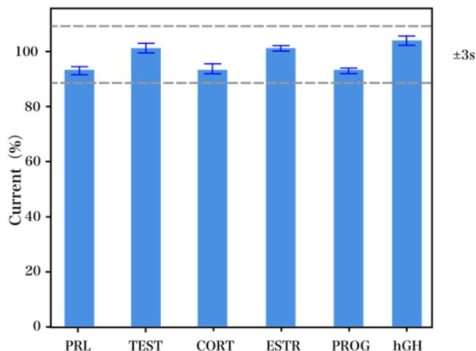
**Figure 3.** Amperometric currents obtained using the AP-anti-PRL-PRL-pPPA/MWCNTs modified GCE after adding cortisol, testosterone, progesterone, oestradiol and human growth hormone (50 ng/mL).
