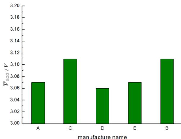
**Figure 9.** The average voltage at the end of discharge,  $\bar{V}_{EOD}$ , for the five manufacturers
