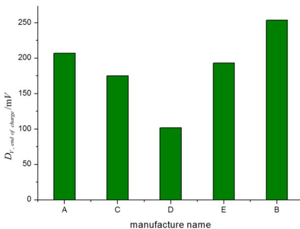
**Figure 10.** Maximum voltage differences at the end of discharge,  $D_{V, \text{end of charge}}$ , for the five manufacturers
