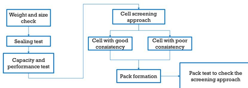
**Figure 2.** Flow of the test procedure in this study
