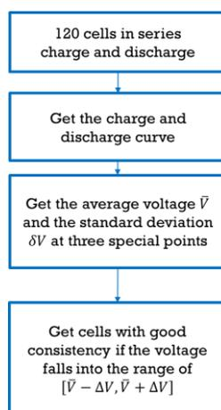
**Figure 4.** The facile screening approach for cell inconsistency
