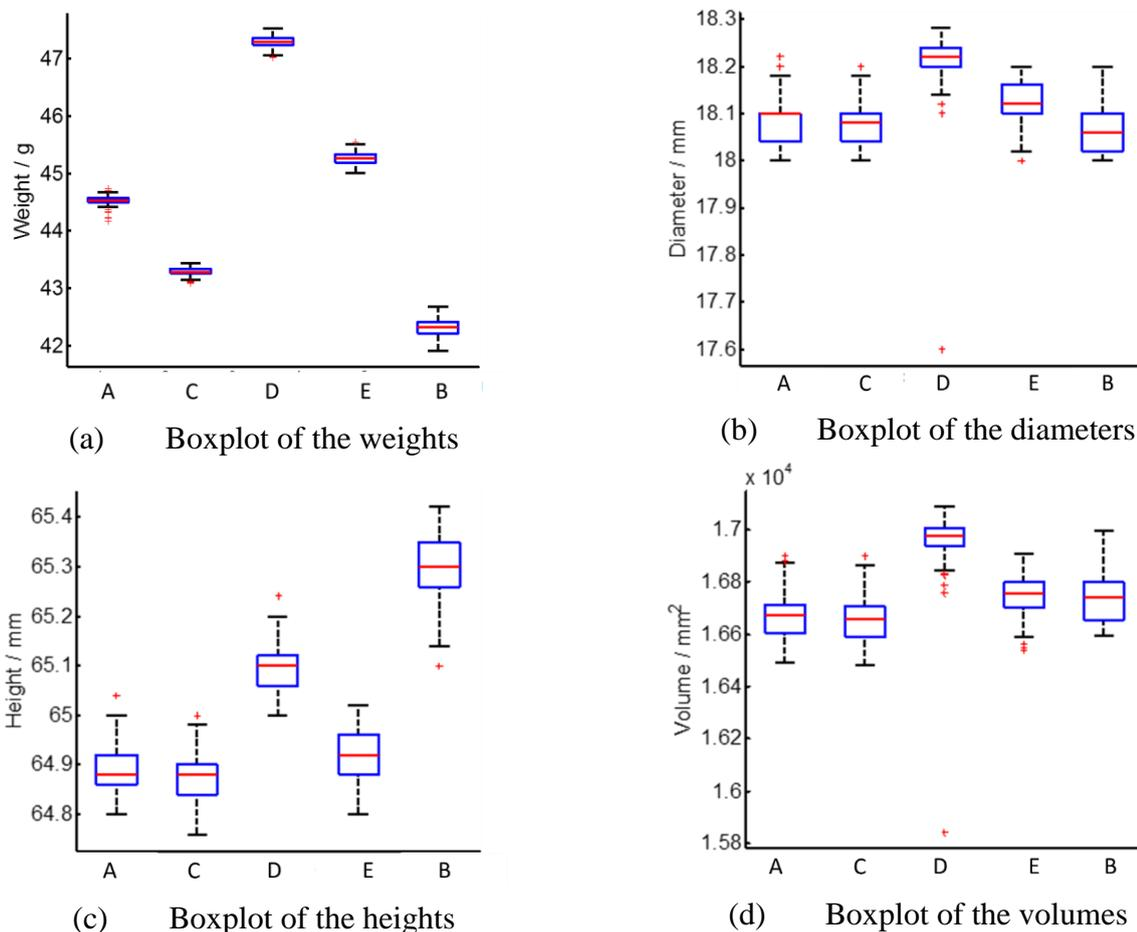
**Figure 6.** Boxplot comparing the inconsistency of the weights and sizes of the cells from the five manufacturers
