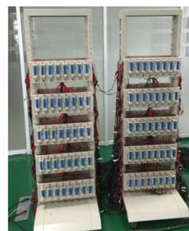
(b) Arbin tester with 120 cells connected in series
