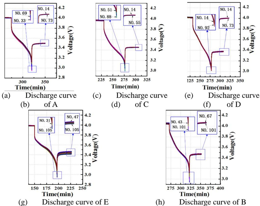
Figure 8. Discharge curves of the individual cells in the 120-cell pack
