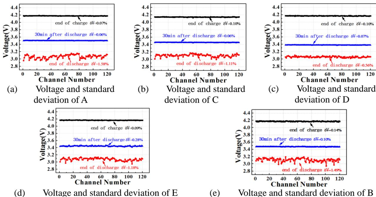
**Figure 11.** Voltage statistics the at the three selected points for the five manufacturers before screening
