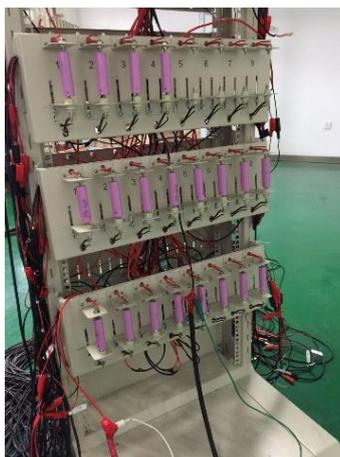
**Figure 5** The pack test setup for verification of the facile screening approach
