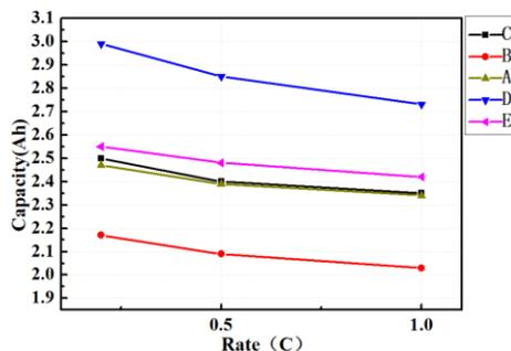
Figure 12. The discharge capacity under different current rates at 20°C
