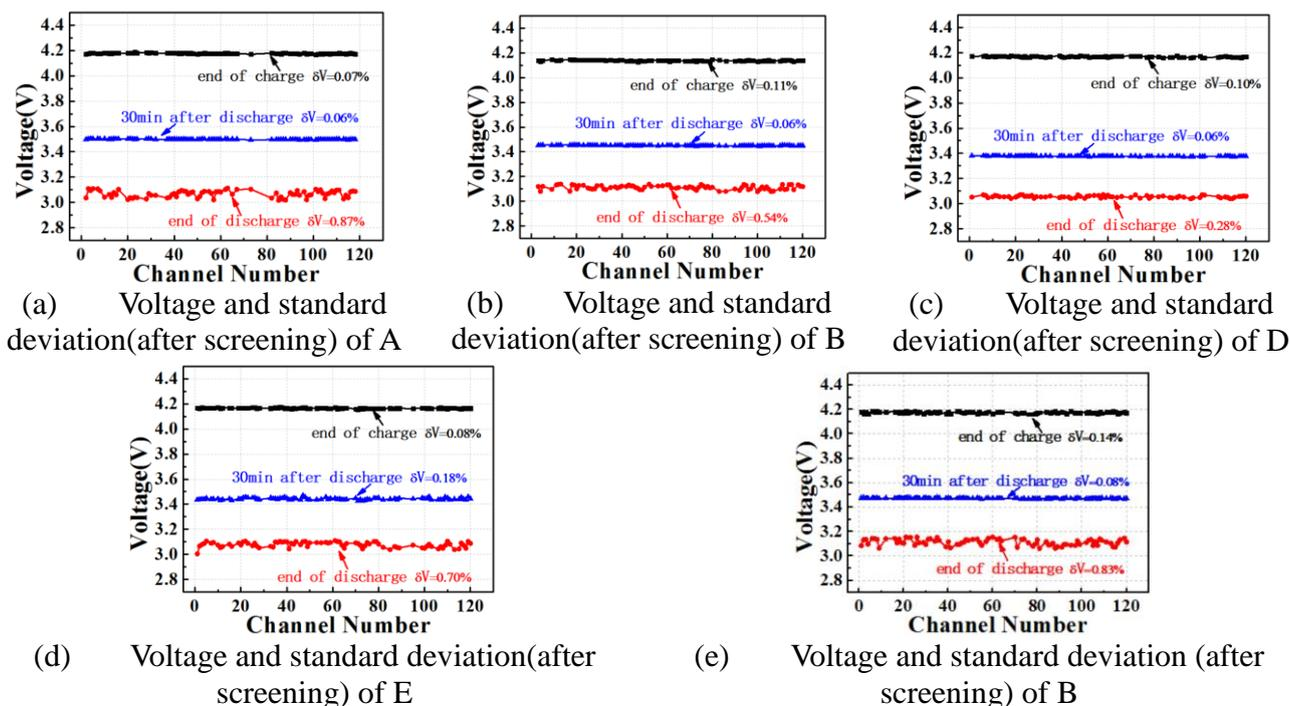
**Figure 15.** Voltage statistics at the three selected points for the five manufacturers after screening
