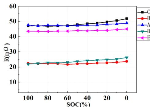
Figure 14. R-SOC diagram of the cell samples for the five manufacturers
