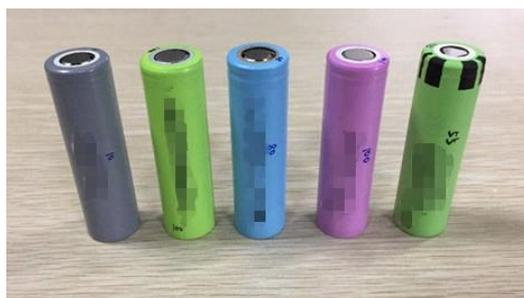
**Figure 1.** 18650 cell samples from five manufacturers
