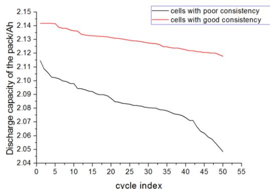
**Figure 16.** Capacity decay for the battery pack, one with good consistency, the other with poor consistency
