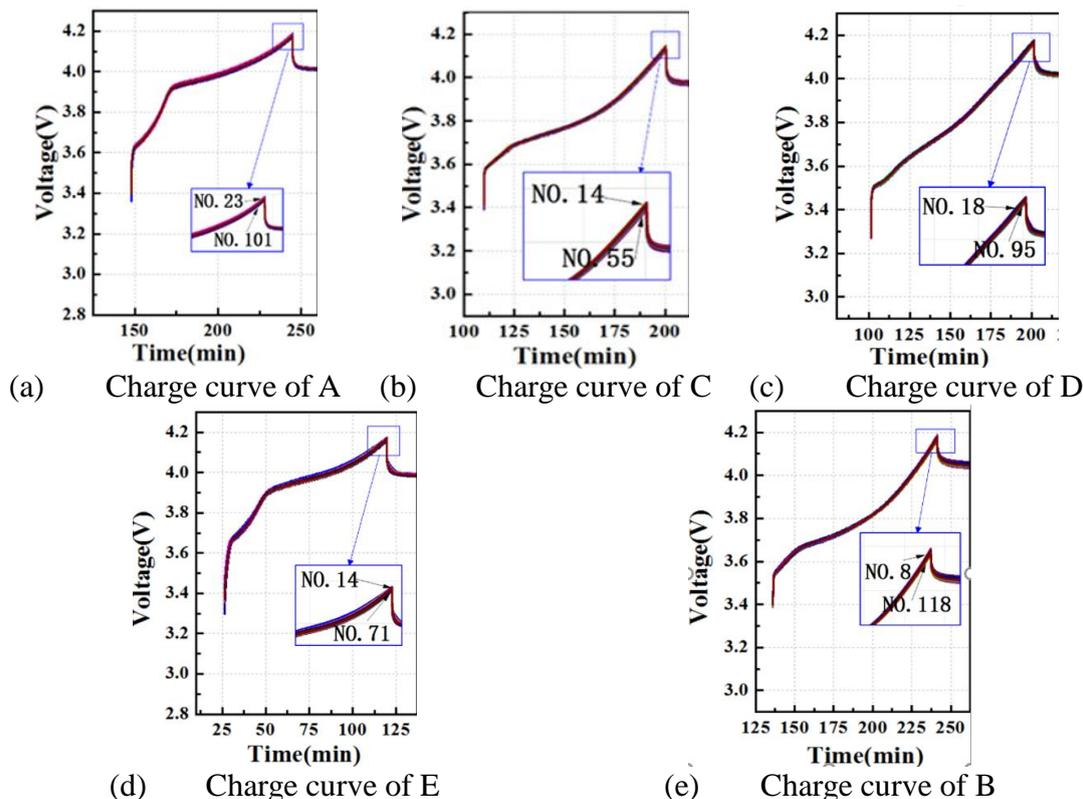
**Figure 7.** Charge curves of the individual cells in the 120-cell pack
