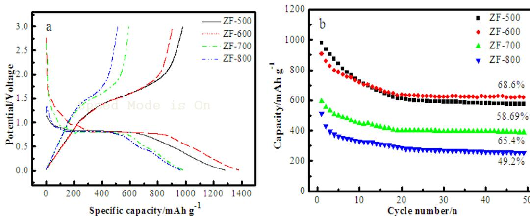
**Figure 3.** Galvanostatic charge-discharge curves(a) and cycling performance(b) of ZF-500, ZF-600, ZF-700 and ZF-800 electrodes
