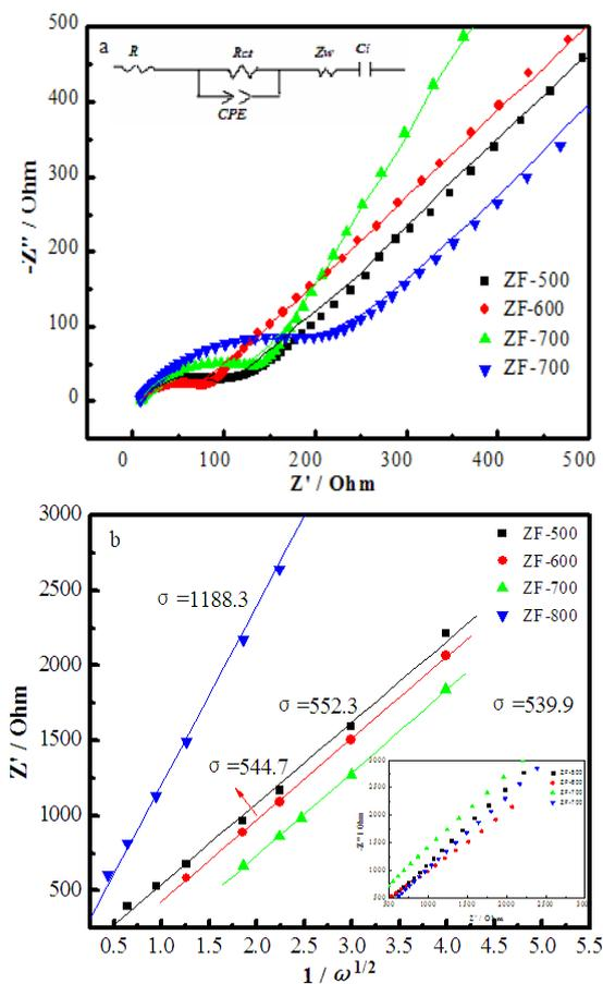
**Figure 5.** Electrochemical impedance spectroscopy and equivalent circuit(a), and the corresponding plots of  $Z_{re}$  vs.  $\omega^{-1/2}$  at low frequency region(b) of ZF-500, ZF-600, ZF-700 and ZF-800 electrodes
