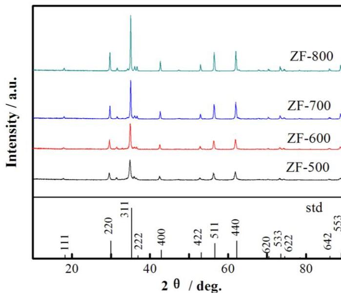
**Figure 2.** XRD patterns for ZF-500, ZF-600, ZF-700 and ZF-800.
