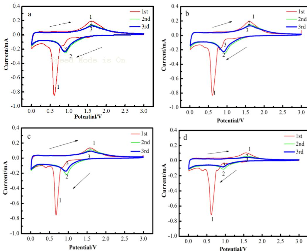
**Figure 4.** The Cyclic voltammograms of ZF-500(a), ZF-600(b), ZF-700(c) and ZF-800(d) electrodes
