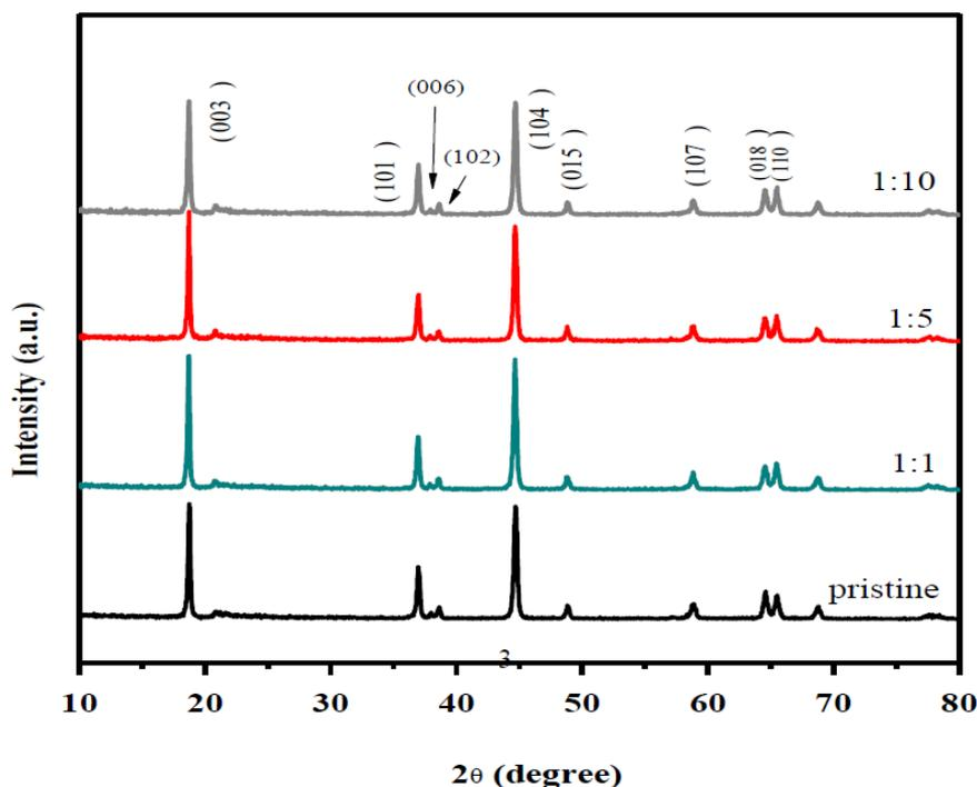
**Figure 1.** XRD patterns of as-prepared LMNCO samples.
