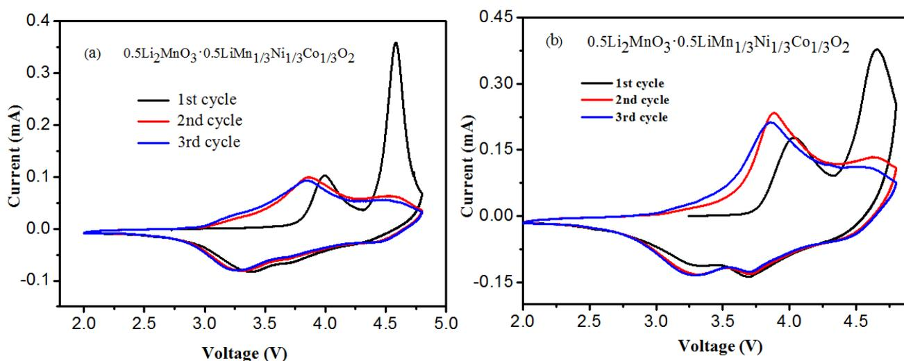
**Figure 6.** CV curves of as-prepared LMNCO samples: (a) pristine and (b) 1:5.
