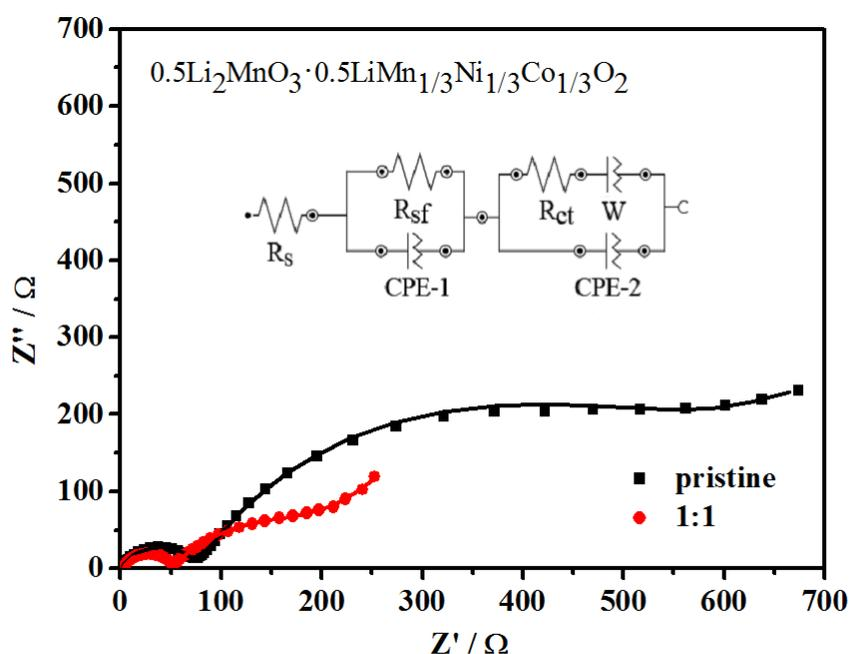
Figure 7. Nyquist plots measured for as-prepared LMNCO samples after 3 cycles.
