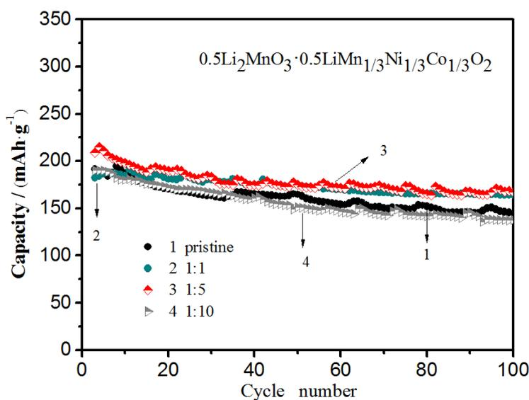
**Figure 5.** Cycling behavior of as-prepared samples.
