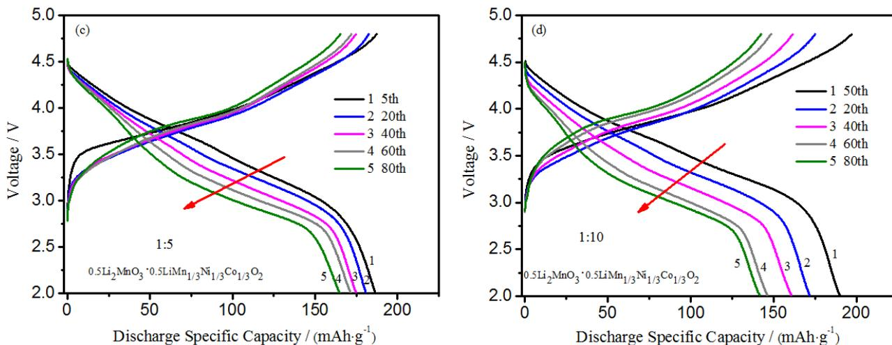
**Figure 4.** The voltage profiles of the as-prepared LMNCO samples at the 5th, 20th, 40th, 60th, 80th cycles
