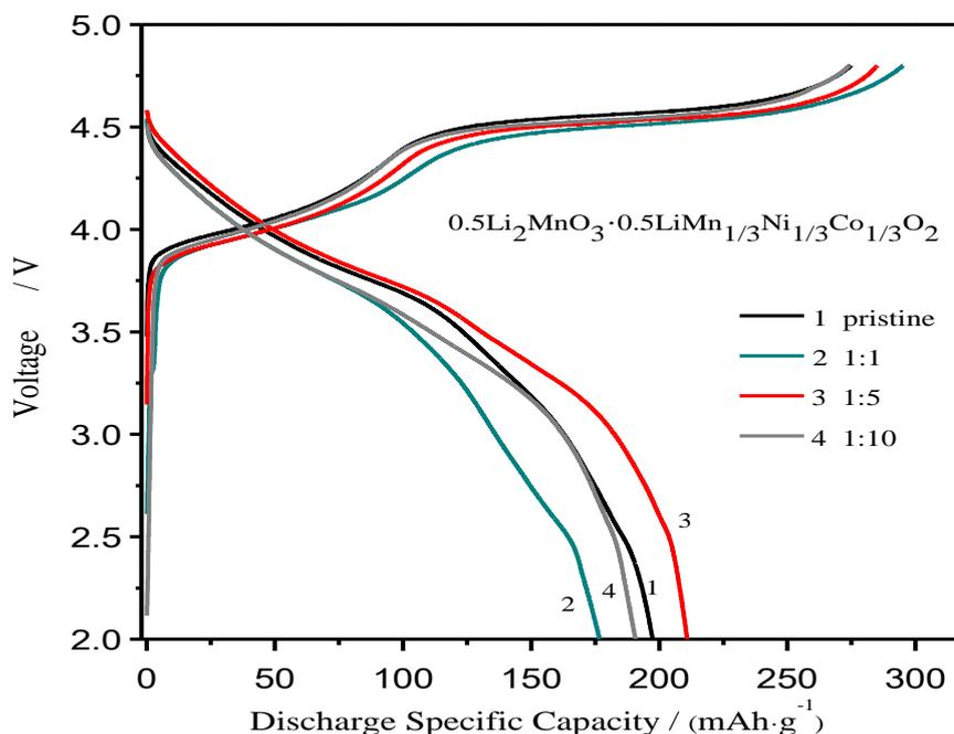
**Figure 3.** Typical initial charge and discharge curves of as-prepared samples.
