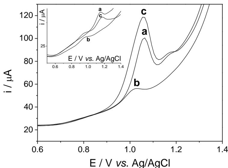
**Figure 5.** Comparison of voltammetric responses of NBV (line a), hydrochlorothiazide (line b) and their mixture (1:1) (line c) recorded at ZrONP-CNT/GCE in 0.1 M H<sub>2</sub>SO<sub>4</sub>. DPV settings same as in Fig. 3. Inset: voltammetric responses recorded in BR buffer pH 4.
