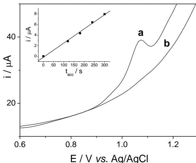
**Figure 3.** Differential-pulse voltammograms of NBV ( $5.0 \times 10^{-7}$  M) at the ZrONP-CNT/GCE in 0.1 M  $\text{H}_2\text{SO}_4$  after preconcentration time of 240 s (a) and without preconcentration (b). DPV settings: pulse amplitude of 50 mV, pulse width of 75 ms and scan rate of  $20 \text{ mV s}^{-1}$ ,  $E_{\text{acc}} = 0 \text{ V}$ . Inset: Influence of the preconcentration time on the NBV oxidation peak current.
