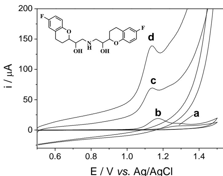
**Figure 2.** Cyclic voltammograms of NBV ( $1.0 \times 10^{-4}$  M) in 0.1 M H<sub>2</sub>SO<sub>4</sub> recorded on different electrode surfaces: bare GCE (a), ZrO/GCE (b), CNT/GCE (c) and ZrONP-CNT/GCE (d). Scan rate: 100 mVs<sup>-1</sup>. Inset: Chemical structure of NBV.
