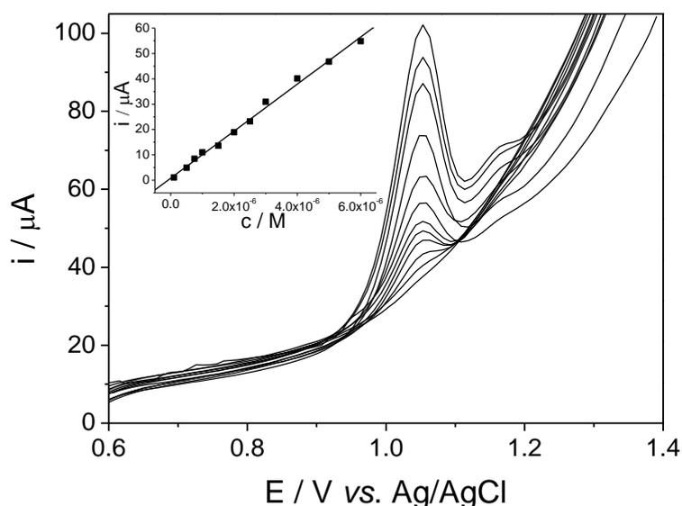
**Figure 4.** Adsorptive stripping differential-pulse voltammograms of NBV at ZrONP-CNT/GCE in 0.1 M  $\text{H}_2\text{SO}_4$  recorded at different concentrations ( $1 \times 10^{-7}$  –  $6 \times 10^{-6}$  M) after preconcentration time of 240 s with corresponding background recording. DPV settings same as in Fig. 3. Inset: calibration graph for NBV quantification.
